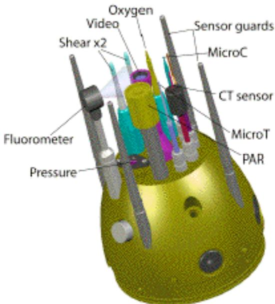
*Figure 5: Sensors on the head of the Air-Sea Interaction profiler.*
