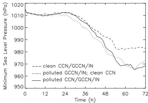
Figure 1: Temporal evolution of the minimum sea level pressure for the MCVs developed in the clean environment (dashed line), the environment with clean CCN profile and polluted GCCN and IN profile (dotted line) and the polluted SAL environment (solid line).
