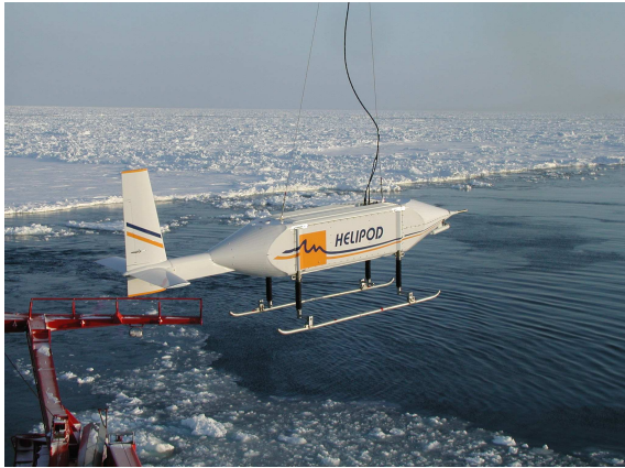
Fig. 1: Helicopter borne turbulence probe Helipod during take off from the research vessel Polarstern.
