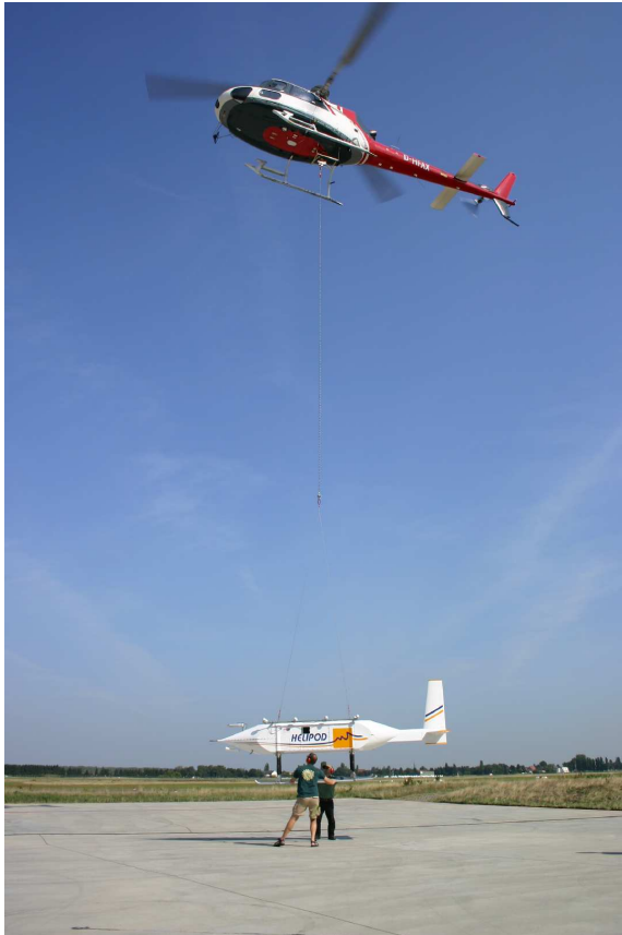
Fig. 1: The turbulence probe Helipod during take off at the research airport Braunschweig.
