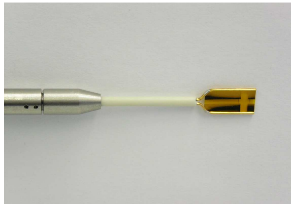
Fig. 4: The fast foil sensor made by Dantec especially for the usage in the M^2AV .
