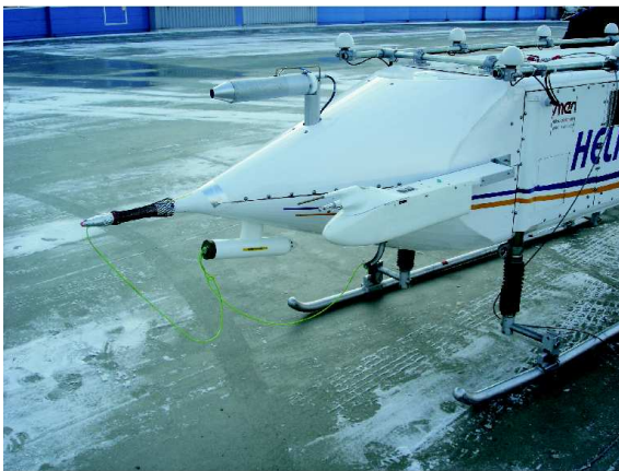
Fig. 6: For a direct comparison of M 2 AV and Helipod data the M 2 AV electronics with the meteorological sensor equipment and the autopilot was mounted to the Helipod during a flight on 27 January, 2006.
