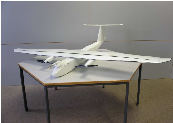
Fig. 1: The autonomous research aircraft M^2AV based on 'Carolo T200'.
