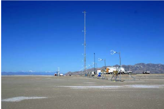
Figure 1. Array of CSAT3 sonic anemometers at the SLTEST site in May, 2005. The instruments were placed forward of a raised causeway, giving about 100 km of unobstructed fetch for winds from Northerly directions.
