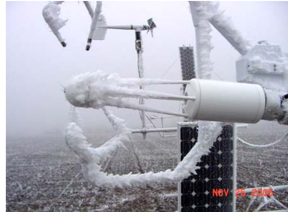
Figure 5. Photograph of an LI7500 sensor head during a frost event in November 2005. Note that all structures are frost covered except for the bottom part of the sensor. The wind direction is on an angle, but mostly from behind the sensor. Photo by Alberto Orchansky.
