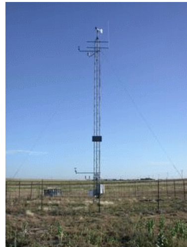
Figure 1. Oklahoma Mesonet 10-m automated weather station tower at Goodwell, Oklahoma.
