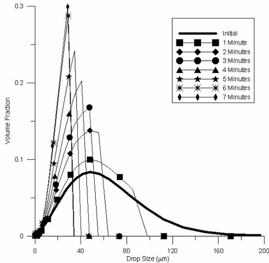
Figure 1: Calculated drop size distributions over time. Drop size distributions are presented for 1 minute intervals for 7 minutes following a source release. The sharp drops are due to the removal of size bins based on settling.
