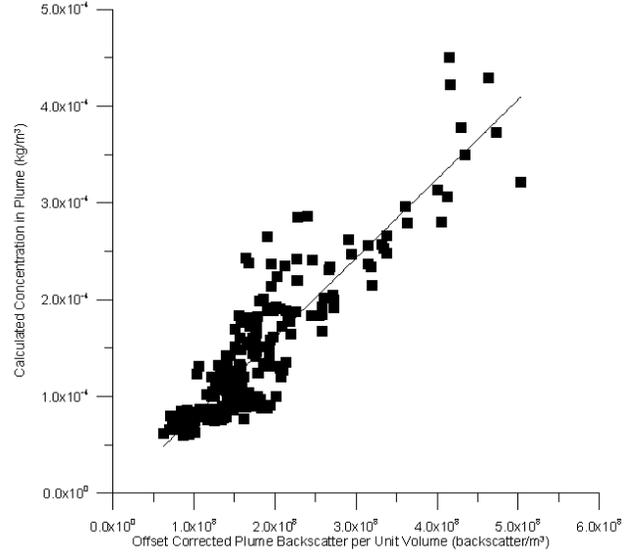
Figure 2: Calculated concentration aloft vs. lidar backscatter per unit volume. All three passes were shifted to a zero intercept to find the relationship. The slope of the linear fit shown on the graph is  $\alpha = 8e-13$ ,  $R^2=0.8$ .
