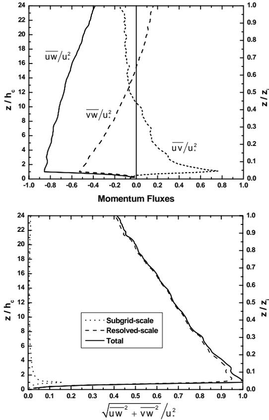
Fig. 2 Vertical profiles of normalized momentum fluxes. In the upper panel, both resolved-scale and subgrid-scale contributions are included.
