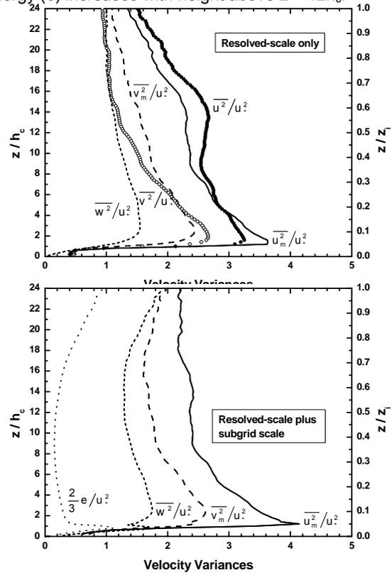
Fig. 3 Vertical profiles of normalized velocity variances. Curves are calculated with the mean wind direction as the streamwise direction at each height. The symbols in the upper panel are calculated in the  $x$  and  $y$  directions.
