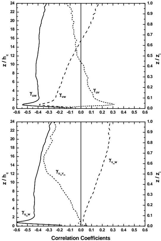
Fig. 5 Profiles of correlation coefficients between velocity components. Upper panel: x-y coordinate. Lower panel: mean wind direction coordinate.
