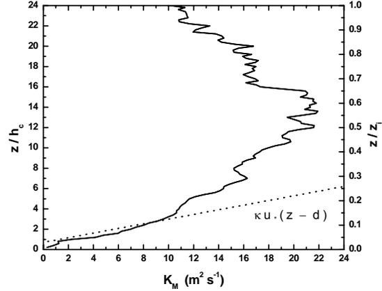
Fig. 9 Profile of eddy-diffusivity for momentum.
