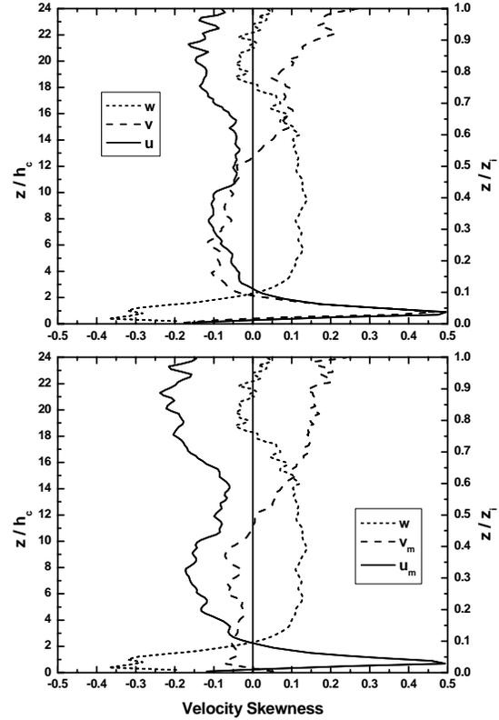
Fig. 6 Profiles of velocity skewness. Upper panel: x-y coordinate. Lower panel: mean wind direction coordinate.
