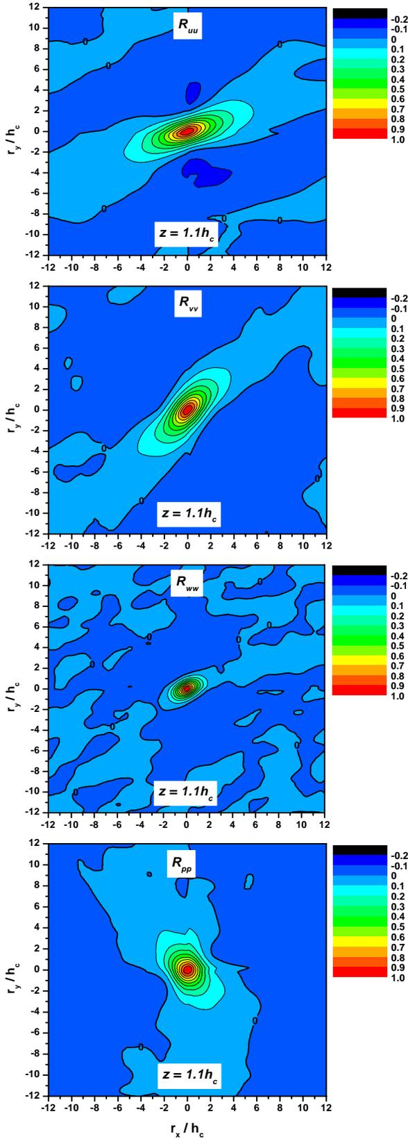
Fig. 13 Two-point auto-correlations with separations in the x and y directions ( $r_z = 0$ ) and the reference near the canopy top.
