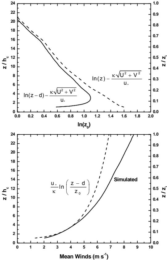
Fig. 8 Estimate of roughness length (upper panel) and the mean wind profiles (lower panel).
