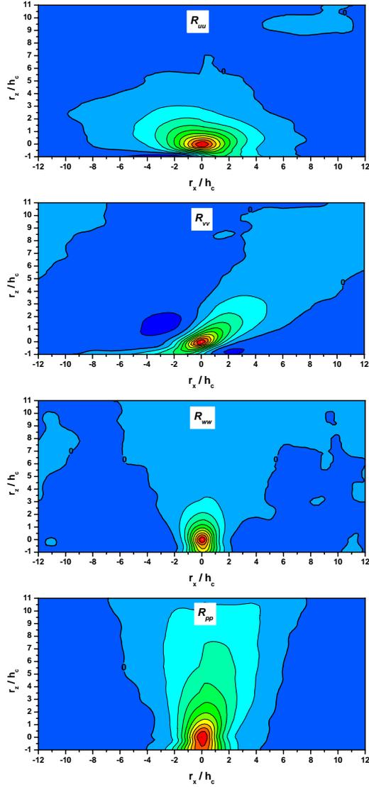
Fig. 11 Two-point auto-correlations with separations in the x and z directions ( $r_y = 0$ ) and the reference near the canopy top.
