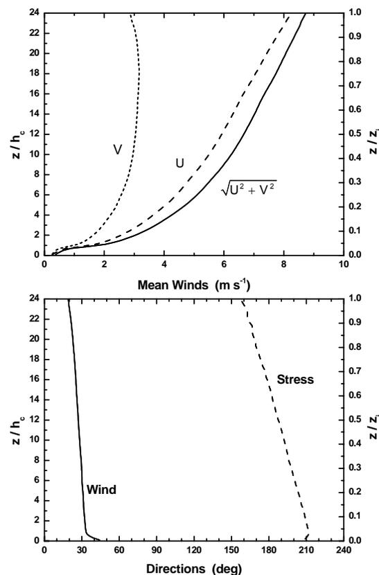
Fig. 1. Vertical profiles of mean wind speeds ( $U, V$ ) in the  $x$  and  $y$  directions and of directions of mean wind and Reynolds stress.
