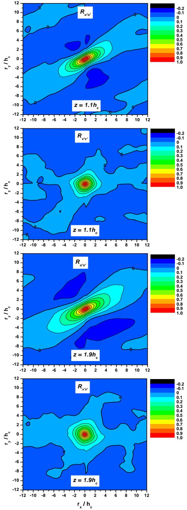
Fig. 14 Similar to Fig. 13 except that  $u'$  and  $v'$  are in a coordinate with the streamwise direction along the mean Reynolds stress direction at each height.
