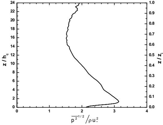
Fig. 4 Profile of standard deviation of fluctuating pressure.
