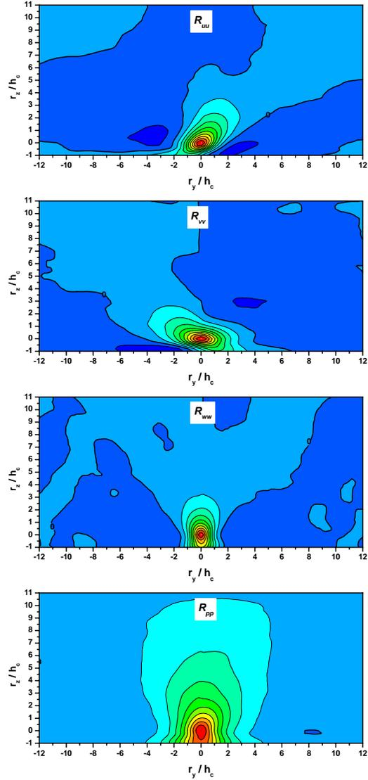
Fig. 12 Two-point auto-correlations with separations in the y and z directions ( $r_x = 0$ ) and the reference near the canopy top.
