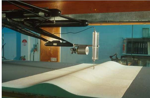
Figure 1: Photo of the wind tunnel configuration in Ayotte and Hughes (2004). Here the hill shape is being measured. Sand covers the hill serving as roughness.
