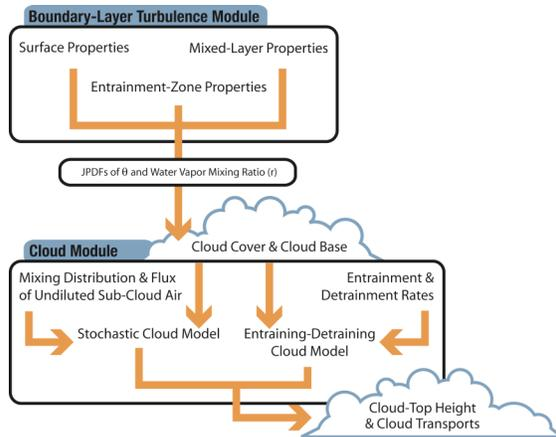
Figure 1. Schematic of the CuP parameterization showing the boundary-layer turbulence and cloud modules. Arrows indicate the flow of information through the parameterization.
