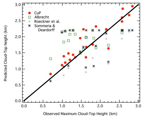
Figure 4. Plot of the Cup (red circles), Albrecht (1981; squares), Roeckner et al. (1996; crosses), and Sommeria and Deardorff (1977; asterisks) predicted cloud-top height vs. observed cloud-top height. The solid line is the 1:1 line.
