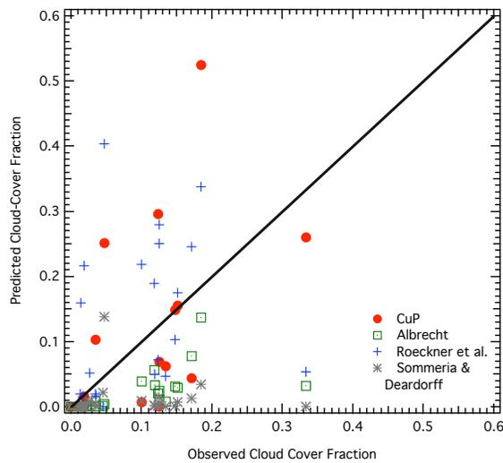
Figure 2. Predicted cloud-cover fraction using the CuP Scheme (red dots), Albrecht (1981; squares), Roeckner et al. (1996; crosses), and Sommeria and Deardorff (1977; asterisks) vs. the observed cloud cover fraction for all BLX96 flight legs. The heavy solid line is the 1:1 line.
