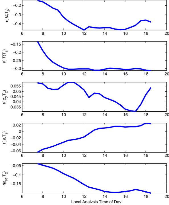
Figure 1: Cross-correlation of  $T_2$  with the various parameters estimated, as a function of time of day.
