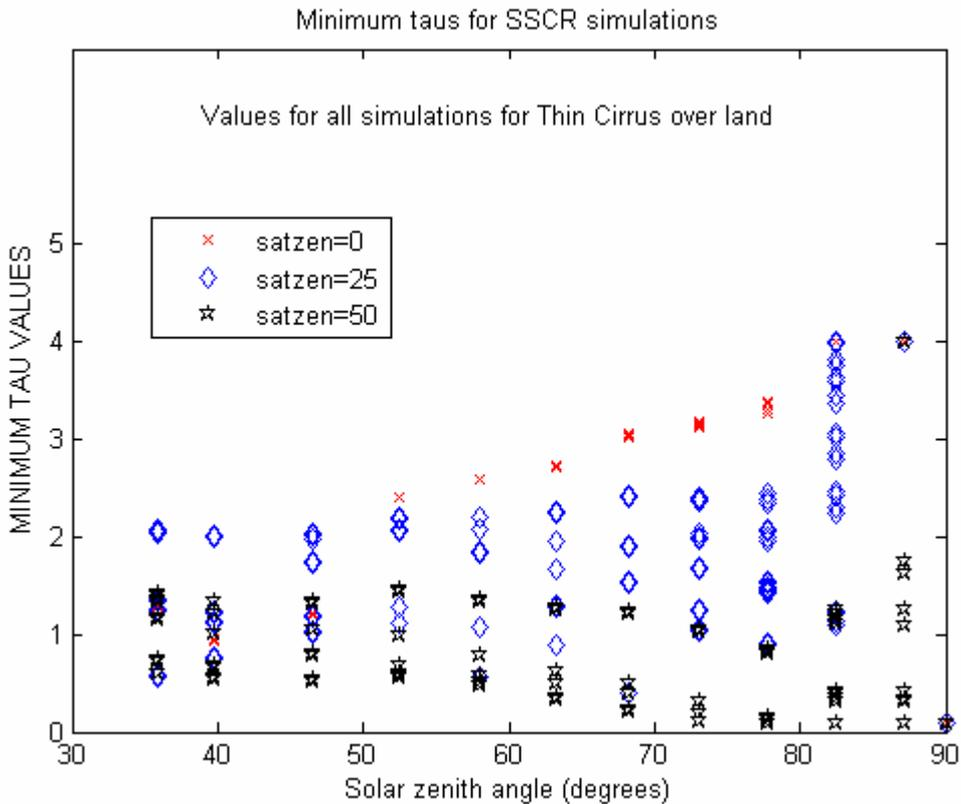
**Figure 3.** Extracted values of the minimum optical thickness for the thinnest Cirrus cloud categories of SCANDIA as simulated by the radiative transfer model SSCR. Simulations were made for an ice cloud over a land surface having a surface reflectivity of 5 %. Results for three different satellite zenith angles (satzen - in degrees) are highlighted.
