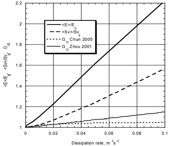
**Figure 17.** Dependences of function  $G_{12}(a_1 + a_2)$ , normalized swept volume and normalized collision efficiency on the dissipation rate for the 10  $\mu\text{m}$ - and 20  $\mu\text{m}$ -radii droplet pair. The collision efficiency increases faster than other quantities. The clustering effect is evaluated using results of Zhou et al (2001) and Chun et al (2005)
