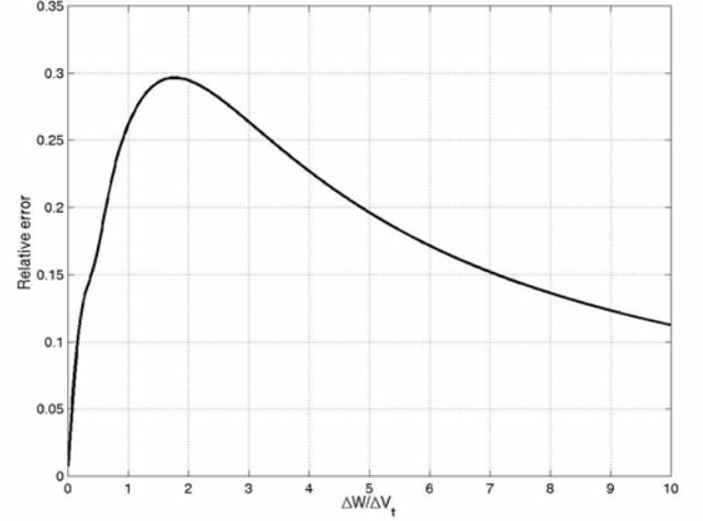
**Figure 18** The value  $(S_v - S_{vadd})/S_v$  as a function the ratio  $\Delta W_{turb}/\Delta V_t$  calculated for 10 and 20 microns radii droplet pair. The calculations were performed under assumption of the Gaussian distribution of relative velocities. The relative error  $(S_v - S_{vadd})/S_v$  becomes significant when both gravity and turbulent effects are important.
