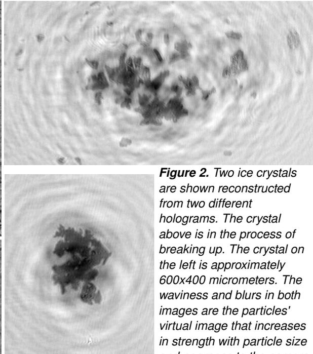
**Figure 2.** Two ice crystals are shown reconstructed from two different holograms. The crystal above is in the process of breaking up. The crystal on the left is approximately 600x400 micrometers. The waviness and blurs in both images are the particles' virtual image that increases in strength with particle size and nearness to the camera.
