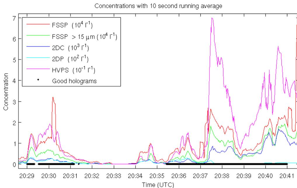
**Figure 4.** Concentrations from other probes on the portion of IDEAS 3 Research Flight 9 in which we process HOLODEC holograms.
