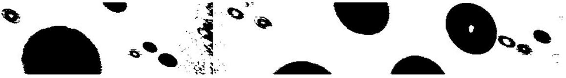
Figure 1: Typical images of natural precipitation drops and spurious images from splashing of drops on the probe. The white space representing distances between images has been eliminated.
