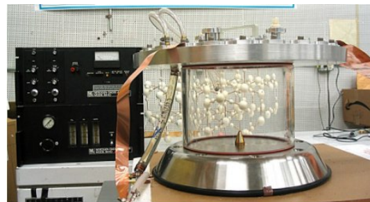
Figure 2. Discharge chamber and \text{NO}_x analyzer used in the study.
