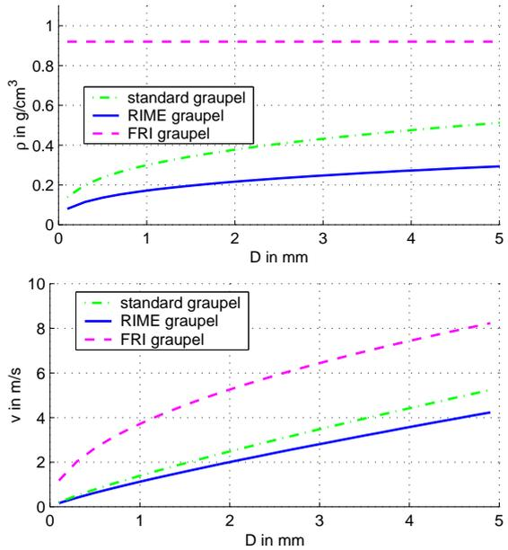
Fig. 1: Density in  $g\ cm^{-3}$  (top) and terminal velocity in  $m\ s^{-1}$  (bottom) as a function of particle diameter in mm for different categories.
