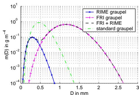
Fig. 2: Mass-size spectra for graupel particles for maritime case 1 at  $y=50$  km,  $x=57$  km,  $z=8$  km and  $t=30$  min. FRI and RIME graupel develop spectra with two distinct modes and combine to a bi-modal spectrum.
