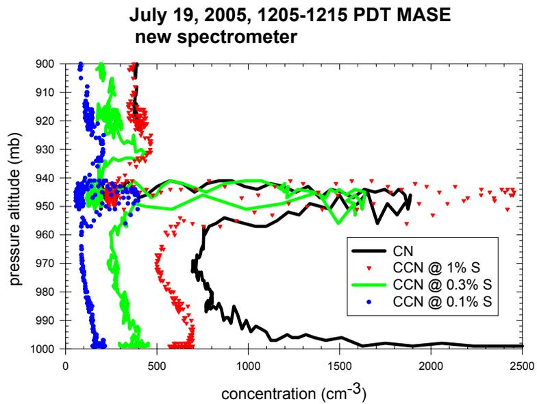
**Figure4.** Vertical profile of CN and CCN at various S off the California coast with low stratus clouds
