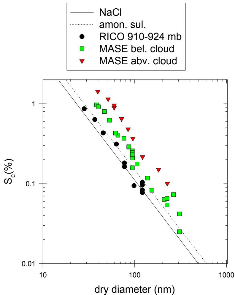
**Figure5.** Size versus  $S_c$  measurements in clean air (RICO) and polluted air (MASE). CCN are larger in more polluted air—i.e., MASE versus RICO and higher altitude in MASE versus lower altitude (see Fig. 3)
