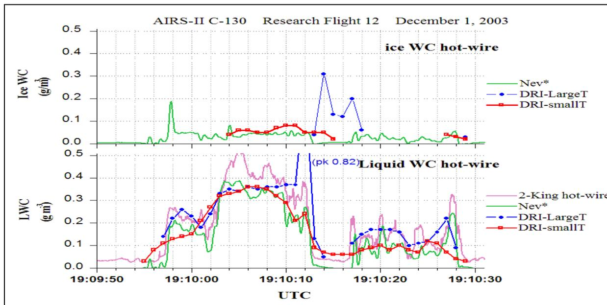
Figure 6. Zooms in on same cloud as Figure 5. Dots mark 1-Hz data, and continuous lines are for high rate (25 Hz) data.
