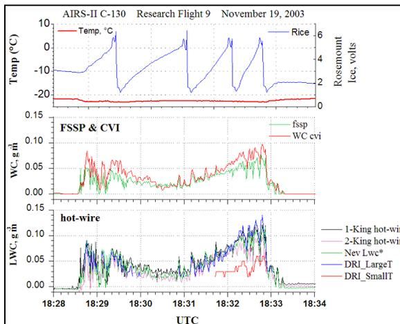
Figure 4. Six minute pass through supercooled water cloud.
