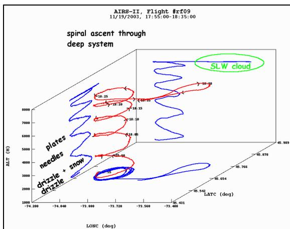
Figure 2. Spiral ascent in deep precipitating cloud system. Blue traces are projections onto horizontal and vertical planes.
