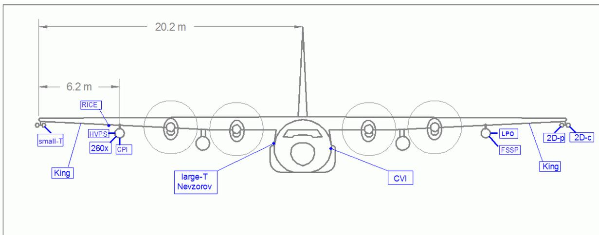
Figure 1. LWC instrumentation on NCAR C-130 during AIRS-2 project.
