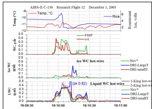
Figure 5. Ninety seconds of data with pass through one small convective cloud.
