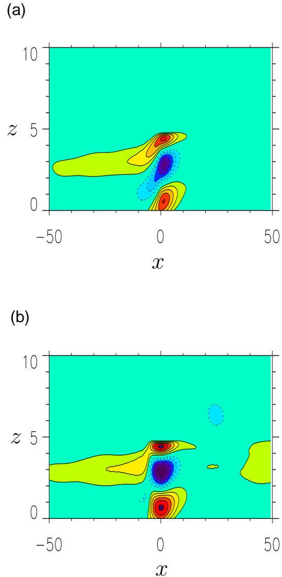
Figure 2: Nonlinear simulation of a gravity wave packet forced by isolated topography: Perturbation streamfunction  $\psi(x, z, t)$  at nondimensional time (a)  $t = 200$  and (b)  $t = 400$ . The contour levels range from negative values of  $\psi$  (shown in blue) through zero (green) to positive values (red).
