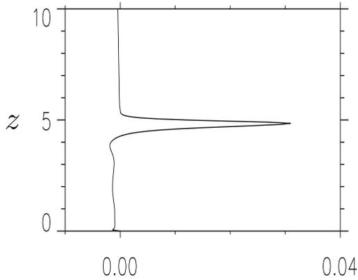
Figure 3: Nonlinear simulation of a gravity wave packet forced by isolated topography: Wave-induced horizontal mean velocity as a function of altitude at nondimensional time  $t = 200$ .
