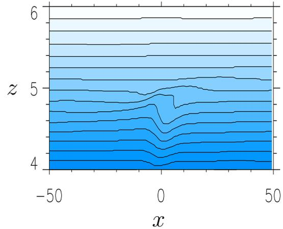
Figure 4: Nonlinear simulation of a gravity wave packet forced by isolated topography: Total density  $\bar{\rho}(z) + \varepsilon\rho(x, z, t)$  at nondimensional time  $t = 200$ . Contour levels decrease with altitude (from dark blue through light blue to white).
