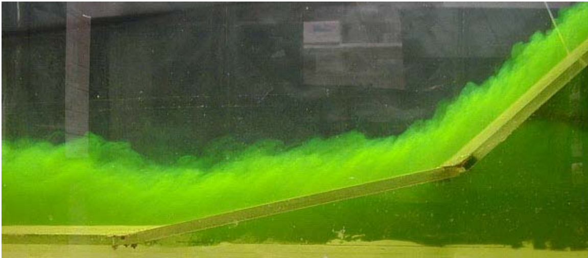
Figure 6: Hydraulic flow on three slopes with angle 0, 10, 35 degrees The source conditions at the gravity current generator are: initial buoyancy jump \Delta b_0 = 30 \text{ cm/s}^2 and the buoyancy flux Q_0 = 45 \text{ cm}^2/\text{s} .
