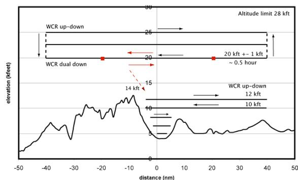
FIG. 1: T-REX UWKA flight-plan schematic with generic cross-mountain flight tracks over the Sierra Nevada and Inyo ranges. Red squares indicate end points of shorter cross-mountain tracks used in a number of research missions, including IOP 11. Gap between the upper and lower set of tracks was necessary to avoid rotor clouds given the Visual Flight Rules (VFR) within the used airspace.
