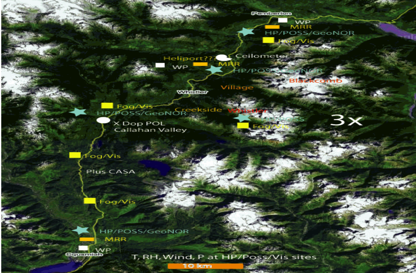
Figure 2: Additional observing systems for operations, Nowcasting and FDP purposes. WP: Wind Profiler (includes RASS); HP: Hot Plate Snow/precipitation sensor; MRR: Microwave Rain Radar; POSS: precipitation- type sensor; GeoNOR: rain Gauge; Fog/VIS: visibility sensors; CASA: potential small footprint radars from the Center for Collaborative Adaptive Sensing of the Atmosphere; X Dop POL: X-band dual polarization Doppler weather radar.
