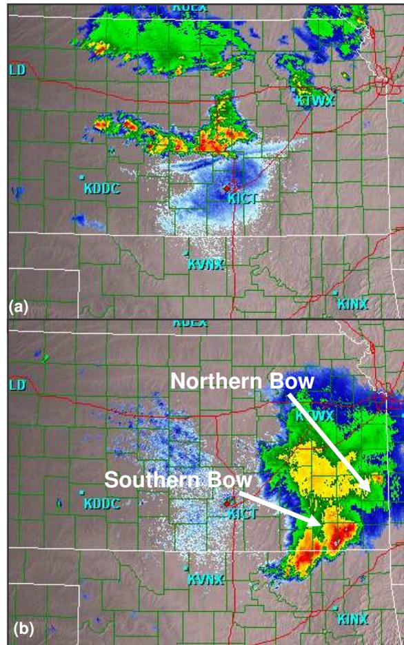
Fig. 3.  $0.5^\circ$  reflectivity image from the WSR-88D at KICT (Wichita, KS) valid at (a) 0648 UTC and (b) 1101 UTC 4 July 2004. The northern bowing segment (eastern Kansas) and southern bowing segment (southeast Kansas) are labeled in (b). State borders (white), interstates (red), county outlines (green), and regional radars (blue) are also identified.
