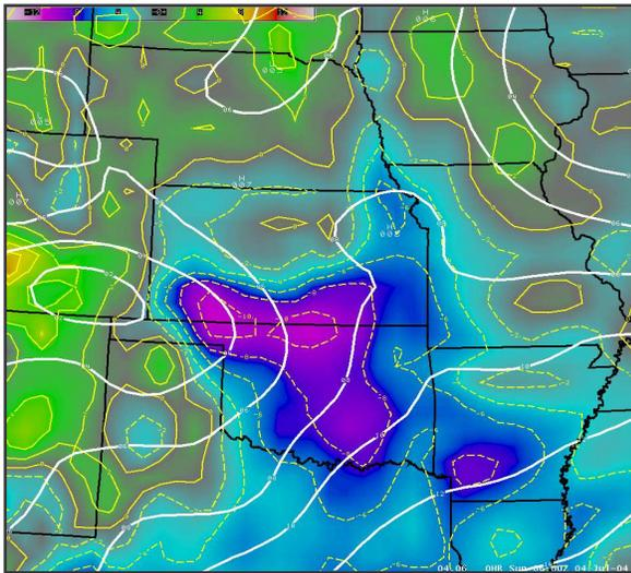
Fig. 2. Surface RUC analysis of mean sea-level pressure (mb) and lifted index ( $^\circ\text{C}$ ) valid at 06 UTC 4 July 2004. The image is of lifted indices (yellow dashed lines are negative values and yellow solid lines are positive values), with mean sea-level pressure identified by white solid lines.
