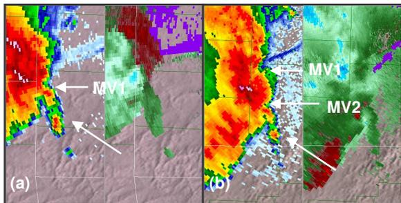
Fig. 6.  $0.5^\circ$  reflectivity and ground-relative velocity two-panels for (a) MV1 valid at 1201 UTC, and for (b) MV2 valid at 1248 UTC. White arrows identify appendages extending from the mesovortices.
