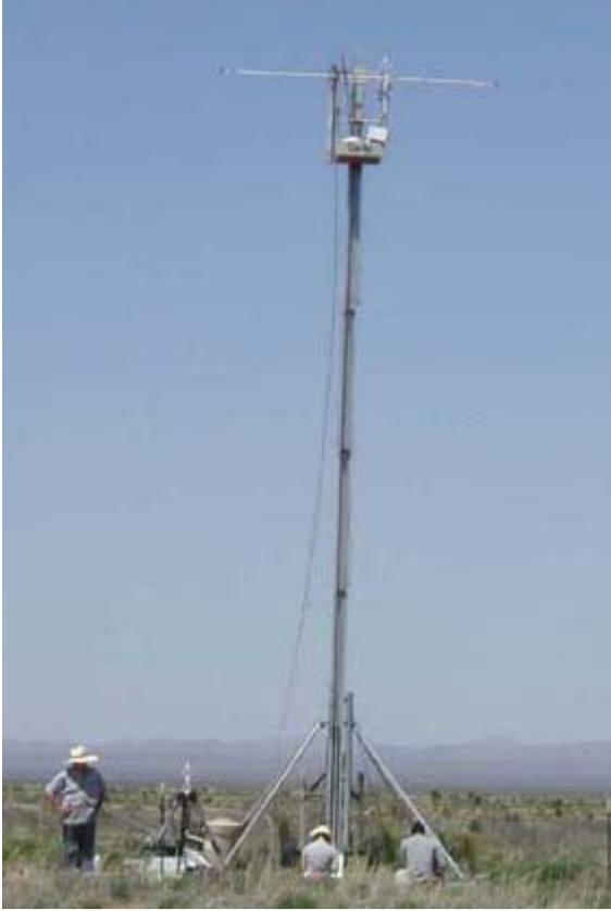
Figure 1: Instrumentation tower. Tower height was 10 meters. At the top a 3D sonic anemometer and finewire thermocouple array took measurements at a rate of 20Hz, and the tracer plume was also release from this height. Microbarographs were located at ground level and a second 3D sonic anemometer was located at 1.5 meters above the ground.
