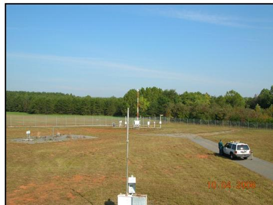
**Figure 3.** View of ASOS from Runway 3, looking north. Remnants of the AWOS-3 visibility sensor suite are located on the graveled area to the left.
