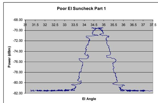
Figure 11: AZ & EL with faulty EL encoders
