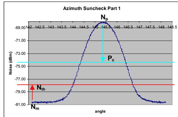
Figure 5: Suncheck Data Thresholds
