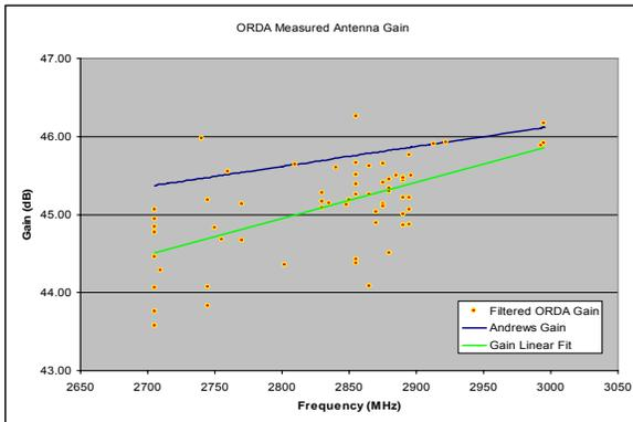
Figure 8: Measured Antenna Gain
