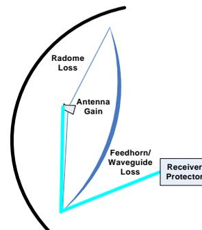
**Figure 1: Antenna Gain Components**
