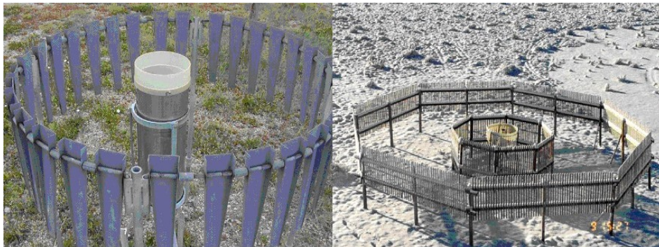
Figure 1 – Left) Single Alter Shield, Right) Double Fenced Intercomparison Reference Shield
