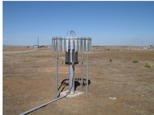
Figure 3 – Example of a three dimensional sonic anemometer deployed inside a single Alter shield with a GEONOR casing.
