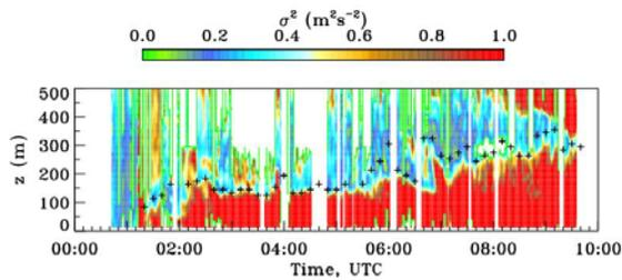
Figure 9. Sample time-height cross sections of the streamwise velocity variance calculated from HRDL vertical-slice scans during night of September 15. Vertical profiles of the streamwise velocity variances were shown to be numerically equivalent to turbulence kinetic energy (TKE) for stable conditions (Banta et al. 2006). The height of the LLJ wind maximum is indicated by plus signs.
