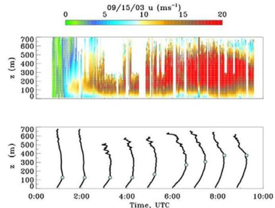
Figure 1. Sample of time-height cross sections of streamwise velocity calculated from HRDL vertical-slice scans during night of September 15; data averaged over (top) 1-min time interval, (bottom) over 1-hour. Velocity profiles were derived from individual vertical-slice scans by sorting the data into 5-m vertical bins. Estimates of the mean and variance were then obtained for each bin. The magnitude range of each wind profile in the bottom panel is 5-20 m s<sup>-1</sup>.
