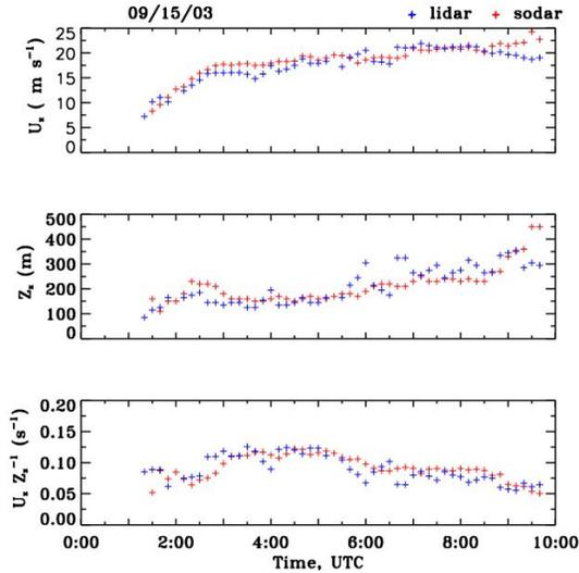
Figure 7. Time-series of the LLJ characteristics determined from HRDL vertical-slice scans (in red) and from sodar measurements with the confidence factor  $\geq 3$  (shown in blue) for the night of September 15.
