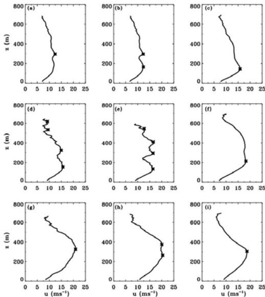
Figure 4 . Sample of the 10-min wind speed profiles with one or more maxima obtained from HRDL vertical-slice scans during the night of September 15. The lowest wind-speed maximum in each case was classified as a LLJ. The second (from the surface) wind-speed maximum in cases (b), (d), (e), and the third wind-speed maximum in case (e) were also classified as LLJs.
