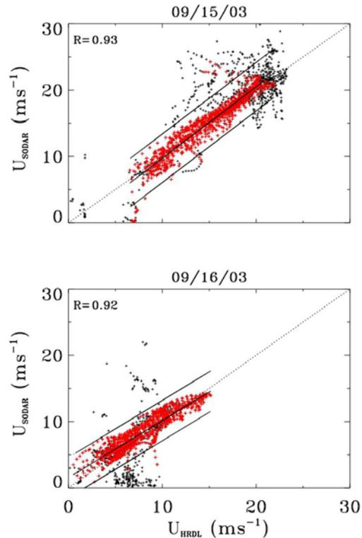
Figure 3. A scatter plots of 10-min, 10-m averaged lidar streamwise velocity and sodar wind speed, obtained for two nights of September 15 (top) and 16(bottom). The middle line in the each plot represents the best-fit linear regression and the upper and lower lines are for  $\pm 1$  standard deviation. The correlation coefficients (0.93-top and 0.92- bottom) were computed only for sodar measurements with confidence factor of 3 or more, which are shown in red on both plots.
