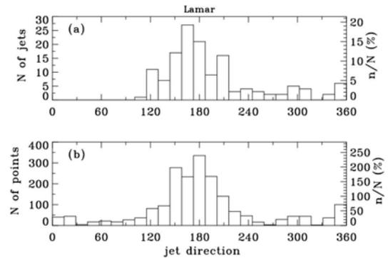
Figure 6. Histograms of jet direction computed from (a) HRDL conical scans and (b) from sonic anemometer measurements at four tower levels for 15-min means. Axis are same as in Figure .
