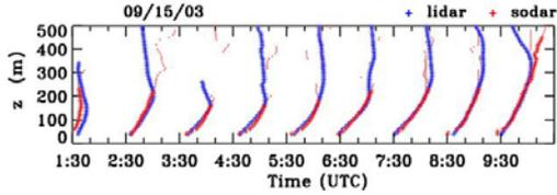
Figure 2. Profiles of 10-min lidar streamwise velocity (blue) and 10-min sodar wind speed profiles (red), for every hour and half from 1:30 to 9:30 during the night of September 15. Red dots show all available sodar data, red pluses are represent sodar data obtained with confidence factor 3 or more.
