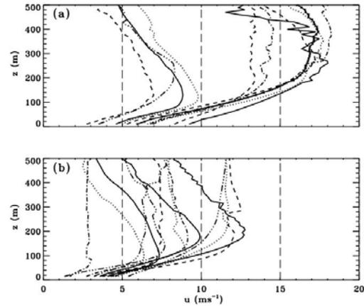
Figure 8 . Profiles of mean streamwise velocity composite for each night of HRDL observations during (a) Lamar-03, and (b) CASES-99 experiments. Different lines in both plots represent different nights; exact dates not important in this context.
