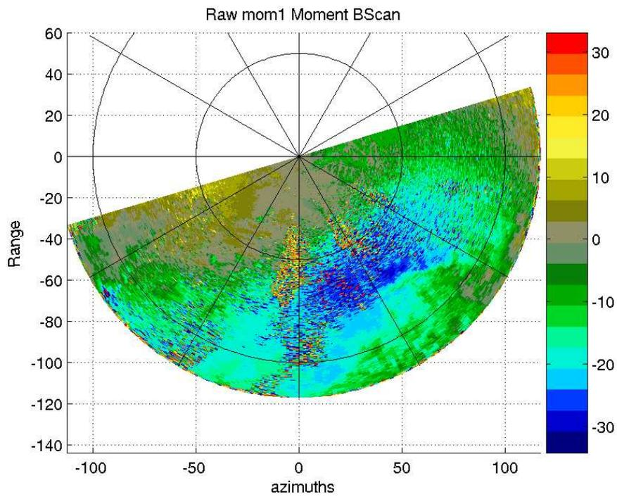
Figure 4: Pulse-pair mean radial velocity PPI plot from data taken on April 5, 2003 at KOUN.
