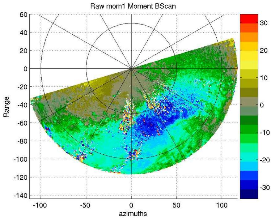
Figure 5: NSPA final mean radial velocity PPI plot from data taken on April 5, 2003 at KOUN. Note, due to a bug, that in cases of very low SNR, velocities are sometimes returned as a missing value (white).
