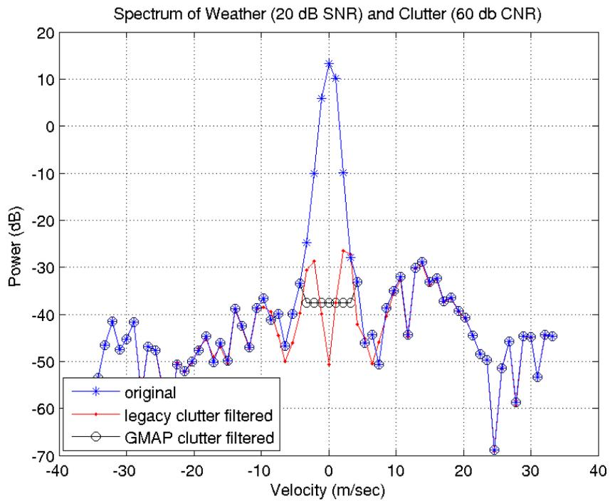
Figure 1: Simulated spectrum of a 20 dB signal to noise ratio weather spectrum centered at 15 m/sec with a 60 dB clutter to noise ratio clutter spectrum centered at 0 m/sec. The original spectrum is shown in blue, the spectrum after the high suppression legacy clutter filter is shown in red, and the spectrum after a high suppression GMAP filter is shown in black. Within the green circle is the clutter power residual after clutter filtering.
