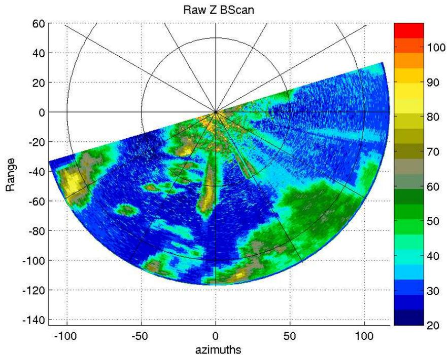
Figure 3: Un-calibrated range-corrected power PPI plot from data taken on April 5, 2003 at KOUN.
