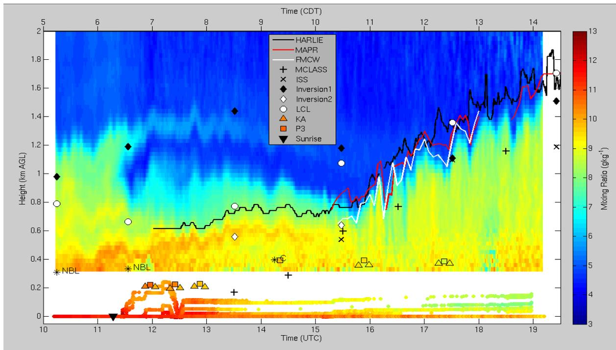
**Fig. 5.** Time series of SRL moisture field obtained from Homestead Profiling Site location shown by dot in Fig. 1. Overlaid are CBL height determined from wind profiler, FM-CW radar and soundings. Sunrise is shown by an inverted triangle. Tethersonde and surface station data are shown beneath the lowest SRL gates.
