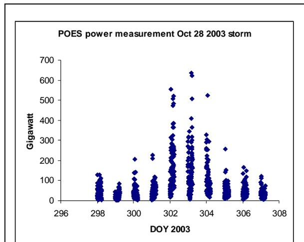
Fig. 5: POES power measurement Oct 28 2003 storm. The power peak was on Oct 30 DOY 303.
