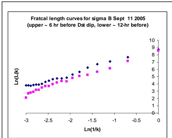
Fig. 3: The fractal length curve of sigma B for two time periods (Sept 11 2005 Dst dip). Upper is the 6-hr period before the Dst dip. Lower is the 6-hr period before that of the upper curve data. The lower curve (slope ~ 2.0) was shifted vertically by about 3 so that it matches the upper curve (slope ~ 1.7) at the origin for easy comparison.
