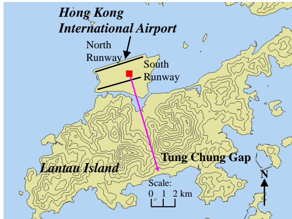
Figure 1 Map of HKIA and Lantau Island (height contours: 100 m). The LIDAR is marked by a red square, with the direction of the Tung Chung Gap vertical scanning indicated by a pink arrow.
