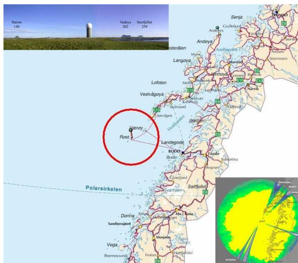
FIG. 1: Radar Røst, its location, and its permanent blockages.
