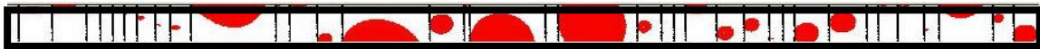
Figure 1: Example of the 2D-C recorded data during T-28 Flight 817 (28 July 2003). The duration for this buffer was 1.003 s and the distance traveled by the airplane during this time is about 100 m.
