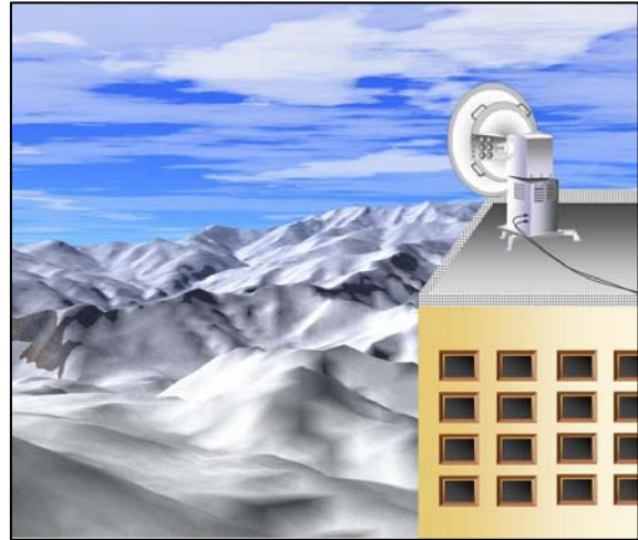
Fig. 4. Schematic illustration of X-POD deployment on the roof of a building for observations over mountainous area.
