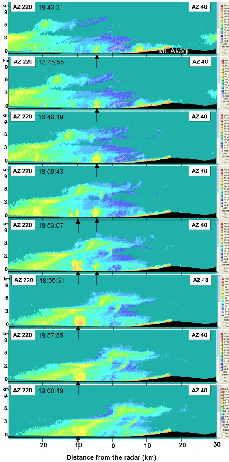
**Fig. 6** Time series of reflectivity RHI scans of 40- and 220-deg azimuth on 01 October 2006. The arrows indicate the quasi-stationary embedded convective cells. The terrains (shadow) are also indicated.
