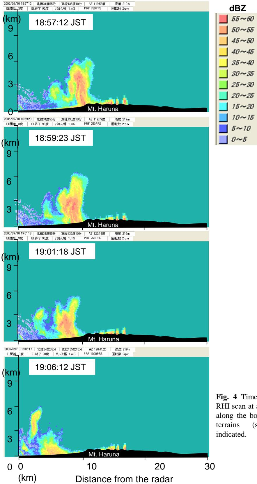
**Fig. 4** Time series of reflectivity RHI scan at azimuth angle 300-deg along the bold line in Fig. 3. The terrains (shadow) are also indicated.
