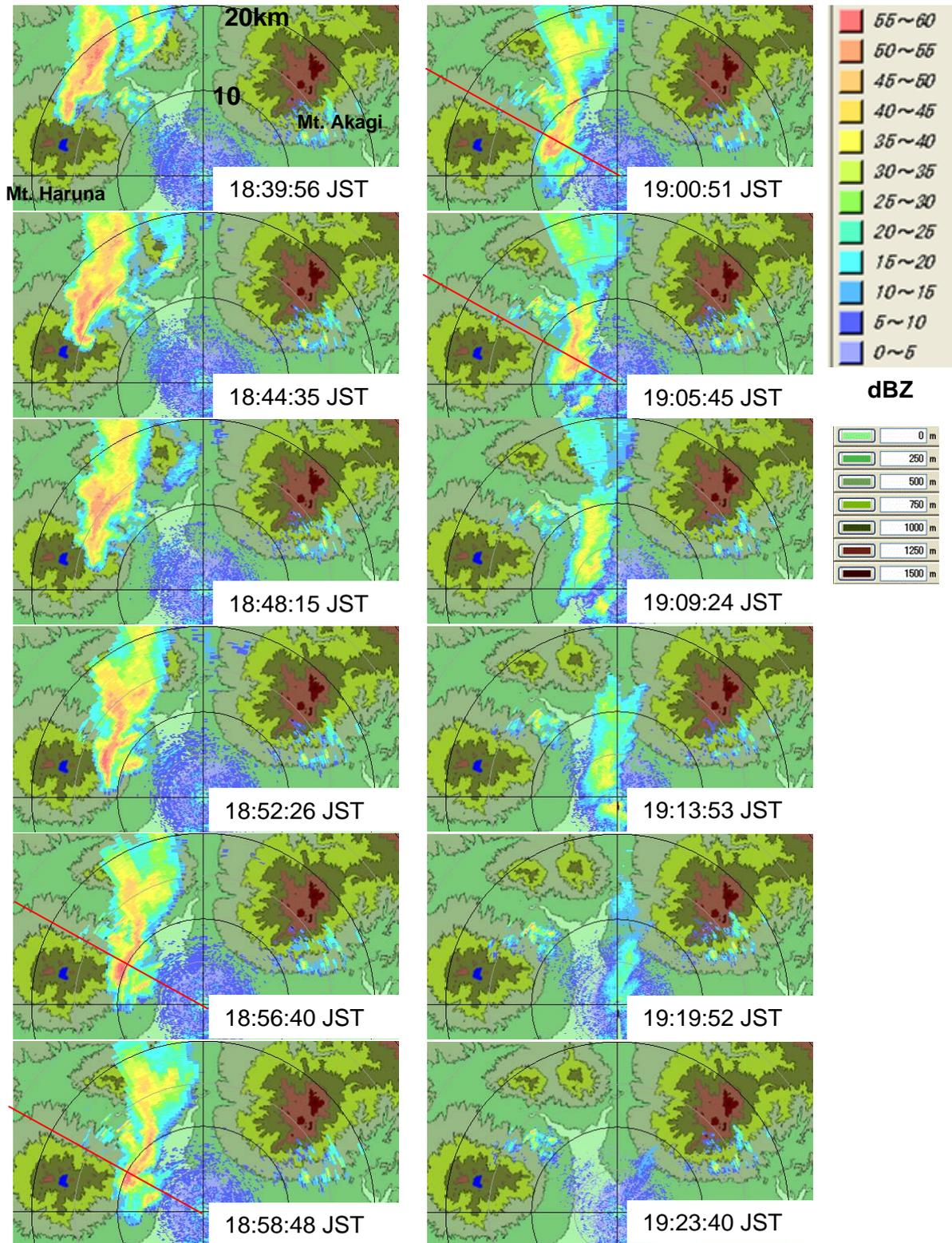
**Fig. 3** Time series of reflectivity PPI scan at elevation angle 5.0 on 10 September 2006 . Terrain contours (intervals of 250 m) are superimposed. The RHI scan beams are indicated by red lines (see Fig. 4).
