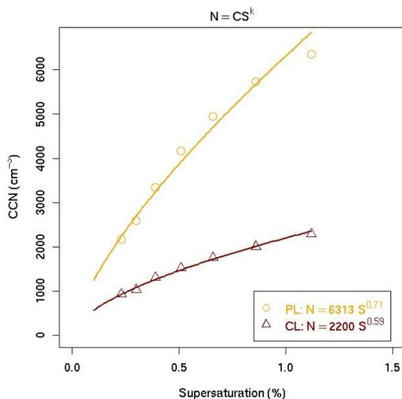
**Figure 10** – Mean cloud condensation nuclei (CCN) activated by the supersaturation indicated inside the counters of Max Planck Institute for Chemistry installed at the Fazenda Nossa Senhora. The polluted period (PL) is represented by 25 October 2002, and the clean period (CL) by 14 November 2002.
