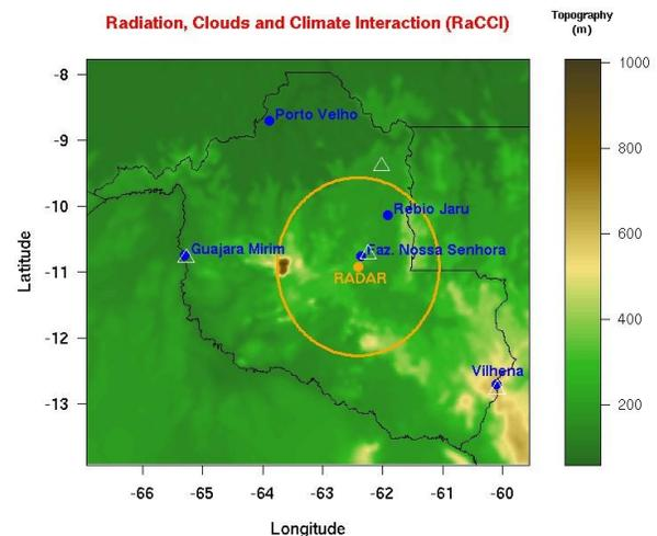
**Figure 1** – RaCCI field campaign instrumentation at Rondonia state, Brazil. The orange site represents the TECTELCOM weather radar location, and blue sites are the radiosonde sites. The Fazenda Nossa Senhora also held the aerosol and CCN counters. White triangles are the BLDN sensors.
