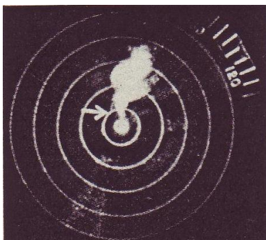
Fig. 3 – Echo associated with hail as observed with an airborne 5.5 cm radar set. The arrow points to the finger considered as an indicator of the presence of hail. [from Battan, 1959]
