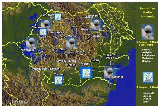
Fig. 1. The SIMIN radar network : 5 WSR-98D S-band radars (un upgraded version of WSR-88D radar used in US NWS network) and 4 C-band radars (2 from EEC – DWSR-2500C type and 2 from Gematronik – METEOR 500C type).
