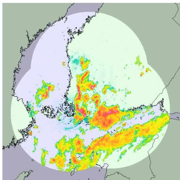
FIG. 4: Composite using MAXIMUM is often preferred in aviation branch; no echo is removed.
