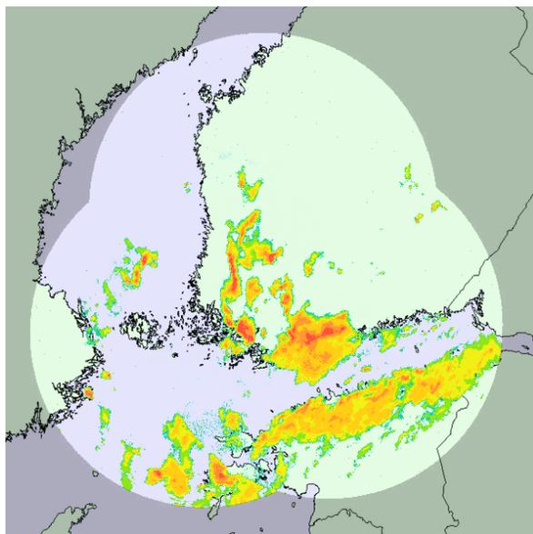
FIG. 2: A three-radar composite applying AVERAGE compositing rule. Korppoo, Vantaa and Ikaalinen radars 9th Aug 2005, 1630 UTC.
