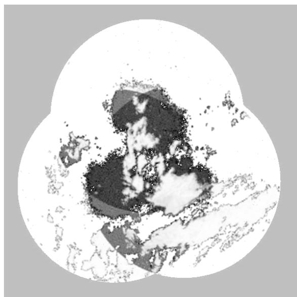
FIG. 3: Deviation (RMSE) of dBZ data originating from three radars. The darkest areas are due to insects which have been removed from the actual product (Fig. 2). Thin contours apparent (also) in single-radar coverage areas originate from bin deviations in subsequent elevations.
