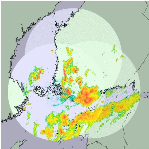
FIG. 5: If radars have varying performance, their contribution in composites can be set accordingly with (quality-) WEIGHTED-AVERAGE. Weighting can be performed at the single-bin level if quality data is available from e.g. anomaly detection.
