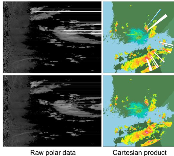
FIG. 7: Correcting attenuation by means of quality-weighted spatial interpolation. Top: attenuation marked; bottom: corrected. Notice that when using this technique it is not that critical *how much* data has been distorted but *where*. (Attenuation has been exaggerated for illustration purpose.)
