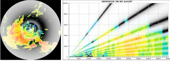
FIG. 1: Visualizing quality: areas of high quality ( $q$ ) are rendered with clear colors. In this example,  $q$  is a degree of measurement representativeness motivated by, but not equivalent to, actual (narrower) beam power distributions.
