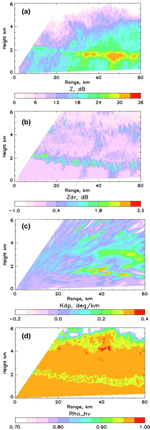
**Fig. 2:** RHI scan taken at 19:02 UTC on 30 Nov 2006, over CARE site (at around 30 km range). (a)  $Z_h$ , (b)  $Z_{dr}$ , (c)  $K_{dp}$  and (d)  $\rho_{co}$ . Of the four,  $\rho_{co}$  shows the upper and lower regions of the melting layer most clearly.
