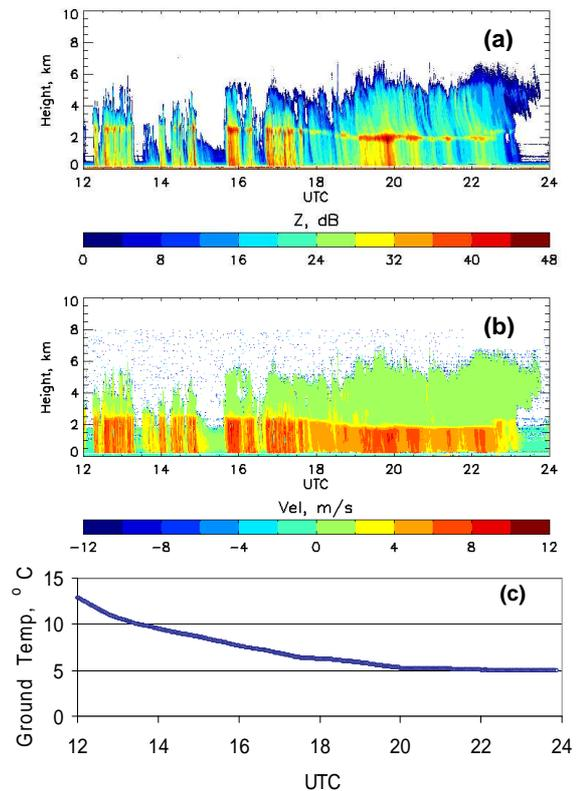
**Fig. 1:** Time series of Z - height profiles (top) and mean Doppler velocity – height profiles (middle) from the VertiX radar, and ground temperature recordings (bottom) at CARE site for the 30 Nov 2006 event.
