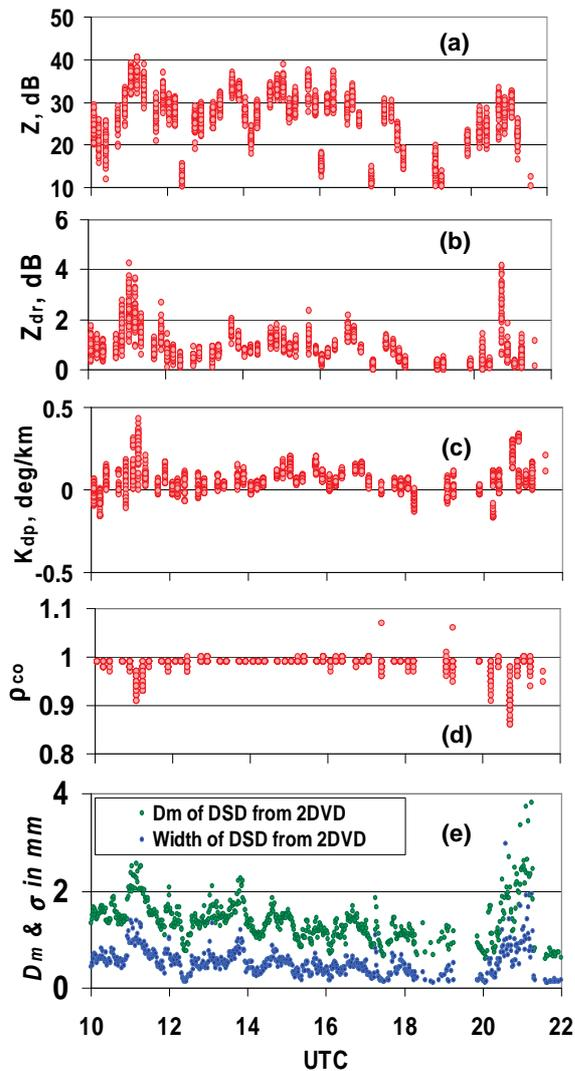
**Fig. 8:** Time series variation of (a)  $Z_h$ , (b)  $Z_{dr}$ , (c)  $K_{dp}$  and (d)  $\rho_{co}$  extracted from the King City radar data over CARE site for the 1 Dec 2006 event. Transition to melting snow occurs just after 20:00, indicated by the high  $Z_h$ , high  $Z_{dr}$  and low  $\rho_{co}$ . The reduction in  $\rho_{co}$  seen at around 11:00 (during the rain period) corresponds to high  $D_m$  (~2.6 mm) and large width (~1.4 mm) of DSD derived from the 2DVD data, both shown in (e).
