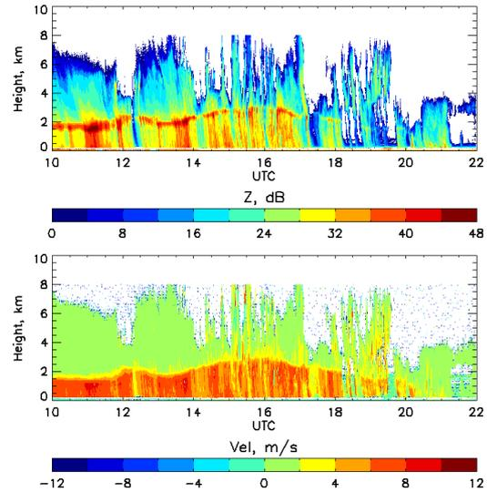
**Fig. 7:** Time series of Z - height profiles (upper panel) and mean Doppler velocity – height profiles (lower panel) from the VertiX radar at CARE site for the 1 Dec 2006 event. The bright-band reaches ground level soon after 18:00 UTC. This is consistent with the 2DVD fall velocity data shown in Fig. 6(a), (b) and (c).
