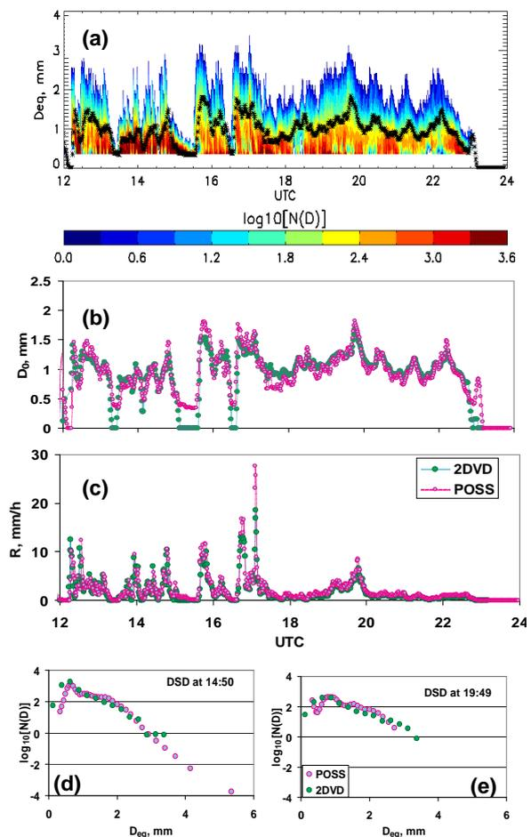
**Fig. 5:** DSDs for the 30 Nov 2006 rain event. (a) DSD time series from POSS, together with the  $D_0$  values superimposed as black stars; (b)  $D_0$  comparisons between POSS and 2DVD; (c) rainrate comparisons between POSS and 2DVD; (d) & (e) DSD comparisons at 14:50 and 19:49. Close agreement between POSS and 2DVD DSDs are seen for this (relatively low  $D_0$ ) event.
