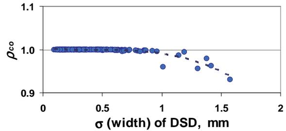
**Fig. 9:** Calculations using the DSD and axis ratios measured by the 2DVD for an event at the CARE site (27 April 2007), showing that  $\rho_{co}$  at C-band could be used to estimate the width of the DSD in heavy rainfall.
