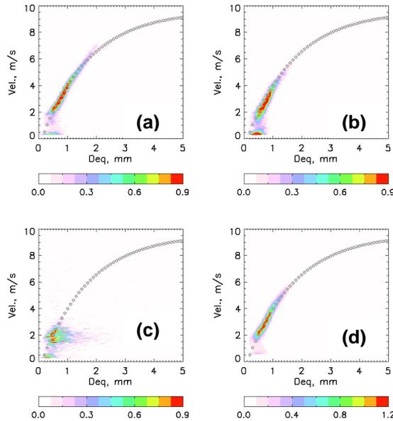
**Fig. 6:** Velocity-diameter variations from 2DVD for the time periods (a) 08:00 – 12:00, (b) 16:00 – 20:00, (c) 20:00 - 24:00 on 01 Dec 2006 and (d) for the entire event on 30 Nov 2006. Color scale represents  $\log_{10}$  of the number of hydrometeors for a given  $D_{eq}$  and a given vertical velocity
