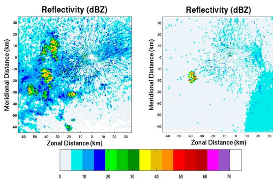
Figure 2: Level-II PPI plots of radar reflectivity from KDDC. The data shown here were taken on two separate days, August 5, 2005 on the left and June 19, 2005 on the right. A clear air reflectivity image of the KDDC coverage region is shown on the right. The same region is shown on the left but with some precipitating cells. It is difficult to distinguish the WTC from the weather in this case. The Level-II data have been filtered by GMAP.
