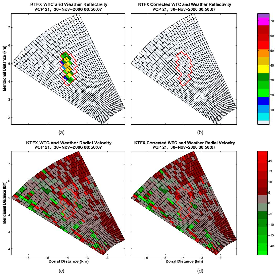
Figure 9: Same as Figure 7 but for KTFX. The WTC and weather reflectivity and velocity PPI plots filtered with OUGMAP are shown in (a) and (c). The results of the 2-D multiquadric interpolation are shown in (b) and (d). The interpolation region is outlined in red.
