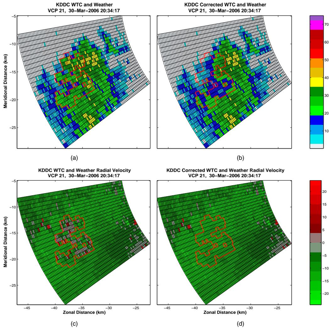
Figure 7: The KDDC reflectivity and radial velocity plots before and after interpolation. The WTC and weather reflectivity and velocity PPI plots filtered with OUGMAP are shown in (a) and (c). The results of the three-dimensional multiquadric interpolation are shown in (b) and (d). The interpolation region is outlined in red.
