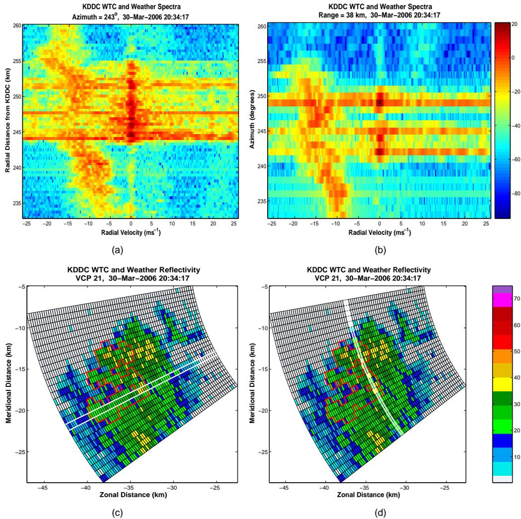
Figure 6: Spectral view of WTC and weather versus range and azimuth. The interpolation technique is well suited for WTC due to the strong spatial continuity of weather. As shown in (a) and (b), the weather signal changes little over approximately 10 kilometers in range and azimuth. Thus the data surrounding the wind farm are appropriate as input for the interpolation algorithm. The regions from which (a) and (b) were created are highlighted white in (c) and (d).
