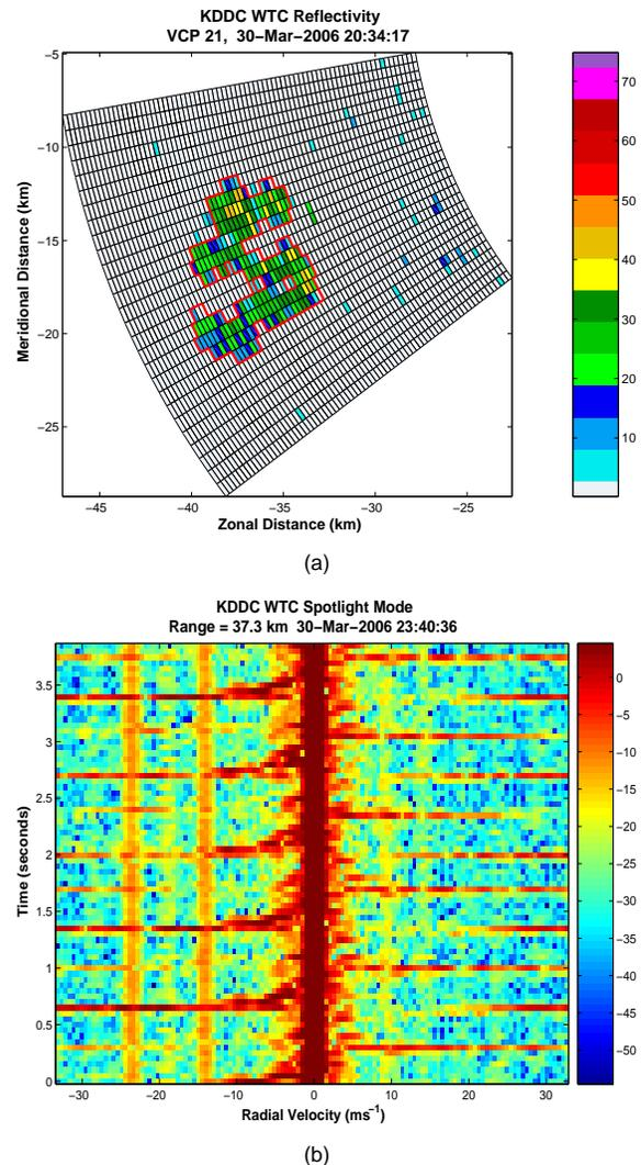
Figure 3: Two methods of data visualization from the KDDC experiment. During the KDDC WTC experiment, data were collected in standard operating modes as well as an unconventional spotlight mode. The  $0.5^\circ$  VCP 21 scan filtered with OUGMAP is shown in (a) with the wind farm region outlined in red. Four seconds of data collected in spotlight mode are shown in (b). The tower is visible at zero velocity while the blades appear as the regularly spaced *flashes*.
