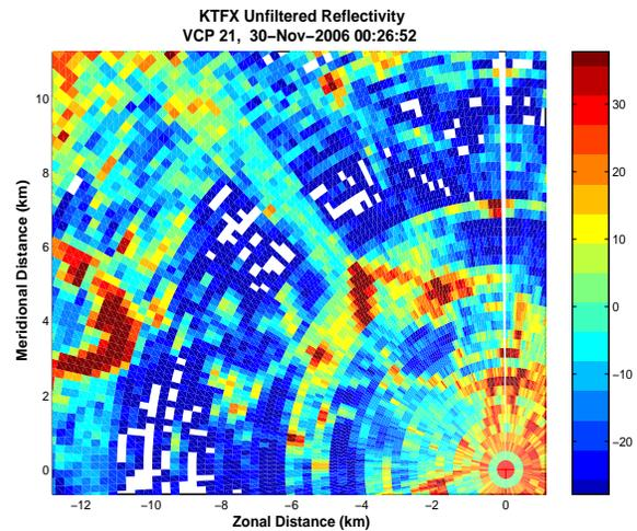
Figure 5: Multi-scatter and multi-trip effects in unfiltered KTFX data. Inter-turbine scatter can be seen in (a) as the *shadow* of higher reflectivity down range from the wind farm. Multi-trip echoes are seen as the area of higher reflectivity exactly twice the radial distance from the radar to the wind farm. The color mapping for this image was altered from the standard for clarity.
