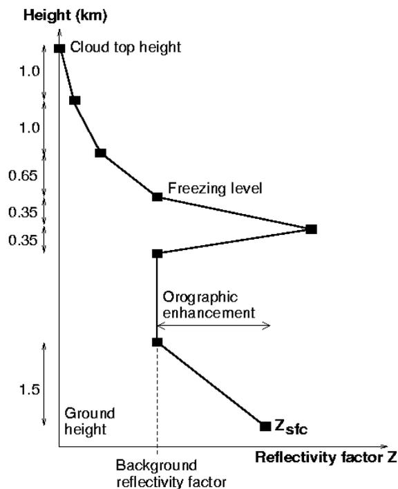
**Figure 1.** Idealised VPR used to correct radar data when a bright band profile is assumed (Kitchen et al 1994).
