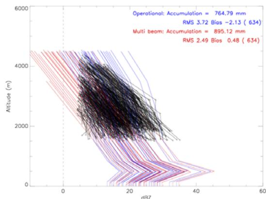
**Figure 7.** Available reflectivity measurements within the rainfall segment circled in Fig 4 and the idealised profiles constructed for each sampling volume using the current operational (blue) and multiple scan (red) VPR correction methods. RMS and bias statistics are computed from the difference between all reflectivity measurements and the corresponding beam-integrated reflectivity across the idealised profile.
