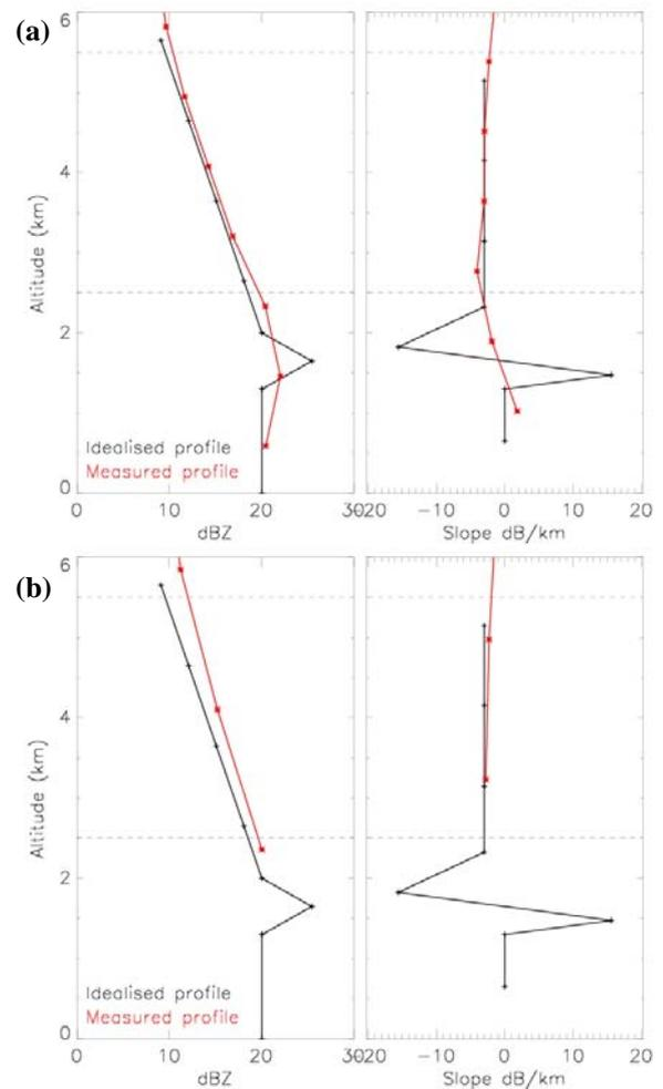
**Figure 3.** Comparison of an idealised VPR and the reflectivity measured by a radar with  $1^\circ$  beamwidth sampling that profile at elevation angles of between  $0.0^\circ$  and  $4.0^\circ$  in  $0.5^\circ$  increments at a range of (a) 100 km and (b) 200 km from the radar. Finite difference slope of the idealised and measured profiles between successive heights are plotted in  $\text{dBkm}^{-1}$ .
