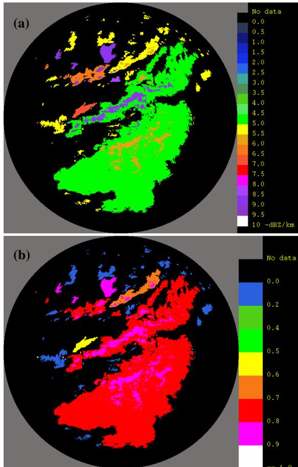
**Figure 6.** (a) Best-fit slope values in each rainfall segment identified in Fig 4(b). (b) Correlation coefficient  $r^2$  for the best-fit slope in each segment. Regions where no local slope could be derived are shown with  $r^2=0.1$ .
