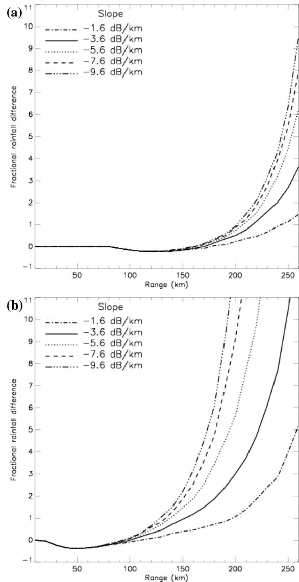
**Figure 2.** Fractional difference between the rainfall sampled by a radar scan (elevation  $0.5^\circ$ ) and the corrected surface rainfall derived using the operational VPR correction scheme assuming different values for the profile slope above the bright band when the freezing level is at an altitude of (a) 2 km and (b) 1 km.
