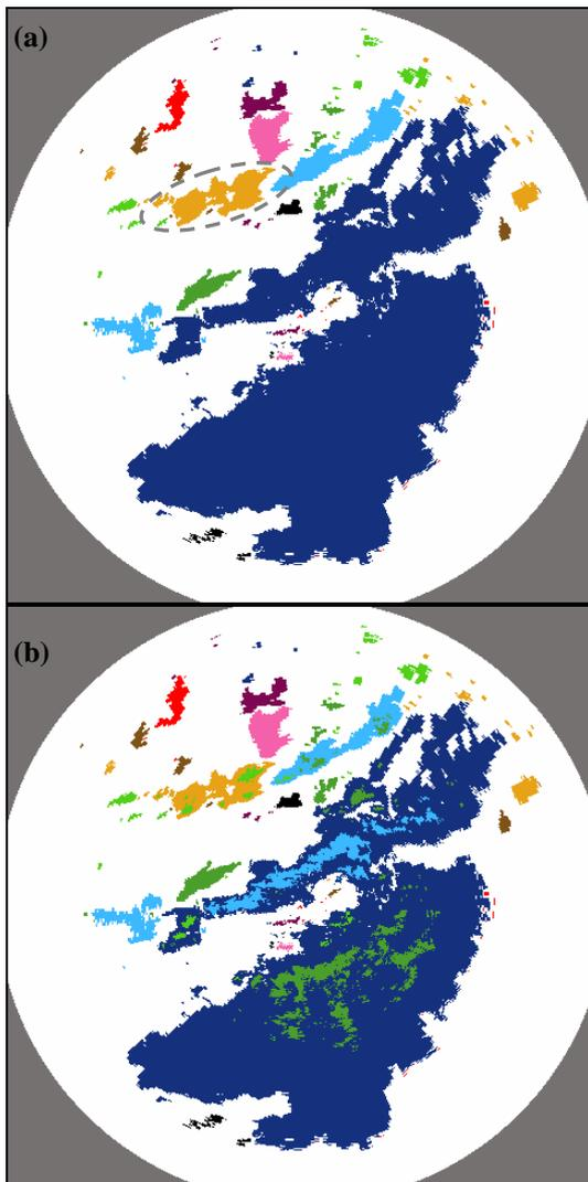
**Figure 4.** Rain segments derived from the lowest usable scan reflectivity measurements. (a) Results of the flood fill algorithm. Different colours represent the distinct segments identified. (b) Larger segments are divided into smaller regions using a method based on the Steiner (1995) criteria with a 30 dBZ threshold.
