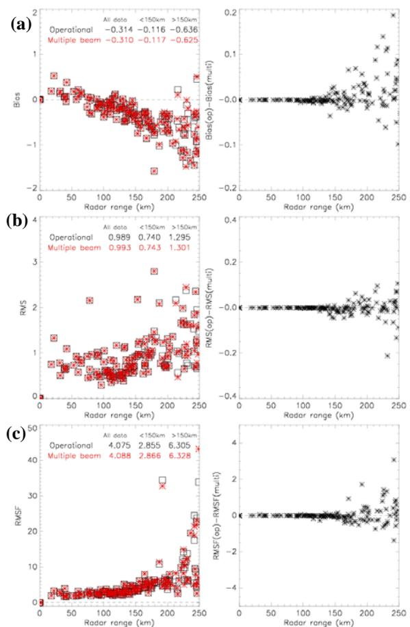
**Figure 9.** Variation of (a) bias (b) root mean square (RMS) and (c) root mean square factor (RMSF) statistics with range from the radar computed from differences between surface gauge measurements of hourly precipitation accumulations and radar data corrected using the operational (black) and multiple scan (red) VPR schemes. The difference between results obtained by each method is also plotted. Positive differences show the multiple scan method to perform better than current operational.
