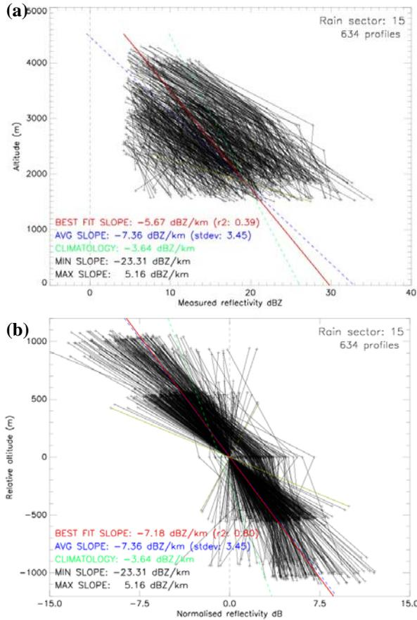
**Figure 5.** (a) Measured reflectivity profiles above the bright band within the rainfall segment circled in Fig 4. Profiles of data measured above the same horizontal location (i.e. radar pixel) are connected. (b) The data are normalised according to reflectivity and beam height. The red line shows the line of best-fit to the data, the blue line shows the average of gradients computed above each individual pixel in the segment.
