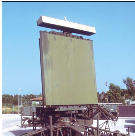
Fig. 1: RAT31SL Phased Array Antenna
