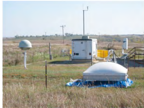
Figure 3: Picture of the UHF boundary layer radar with the ARM site shown in the background.
