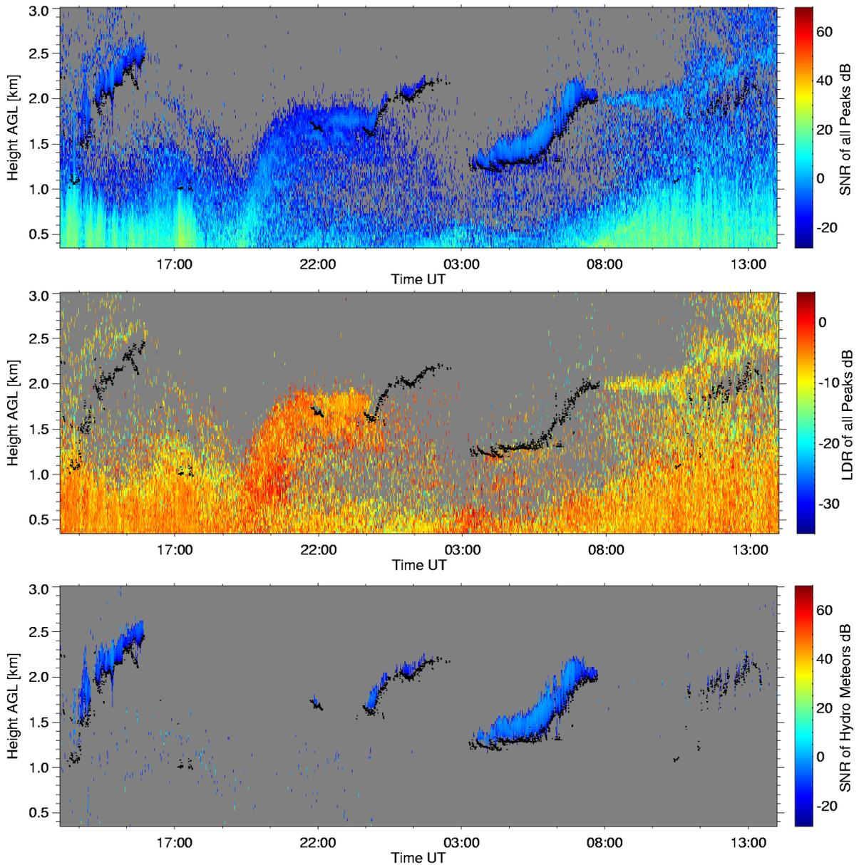
Figure 4: Data measured by the DWD-MIRA36 on 23.05.2007. In the upper picture the SNR of all peaks and in the lowest picture only the hydrometeor peaks are shown. In the upper picture the clouds are hidden in Plankton. Also in the LDR of all peaks (middle picture) its hard to recognize the clouds. The black dots indicate the cloud bases found by a co-located ceilometer. They are in good agreement with the clouds classified by mmclx.
