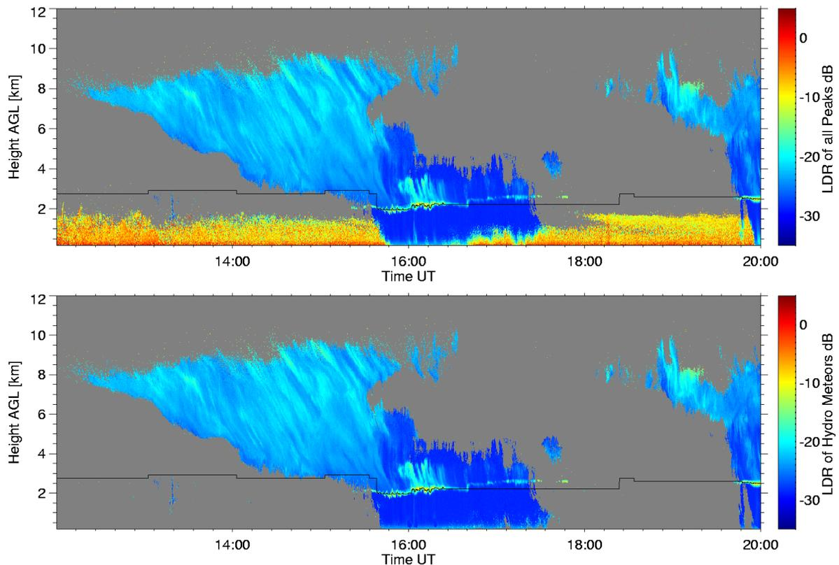
Figure 2: Linear De-polarization Ratio (LDR) from the same measurements as in figure 1 (upper picture: power weighted average of all peaks; hydrometeor peaks).
