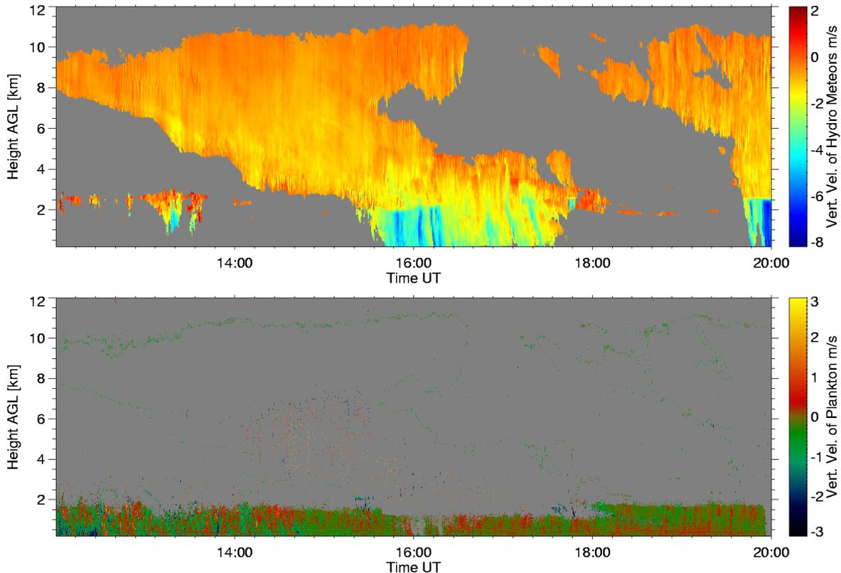
Figure 3: Doppler Velocity of the plankton from the same measurements as in figures 1 and 2. The plankton may be regarded as tracer for the vertical wind turbulence. During strong rain the plankton is covered by the signal from the rain but it is not washed out. During stronger rain the velocity of the plankton could be obtained from the cross channel.
