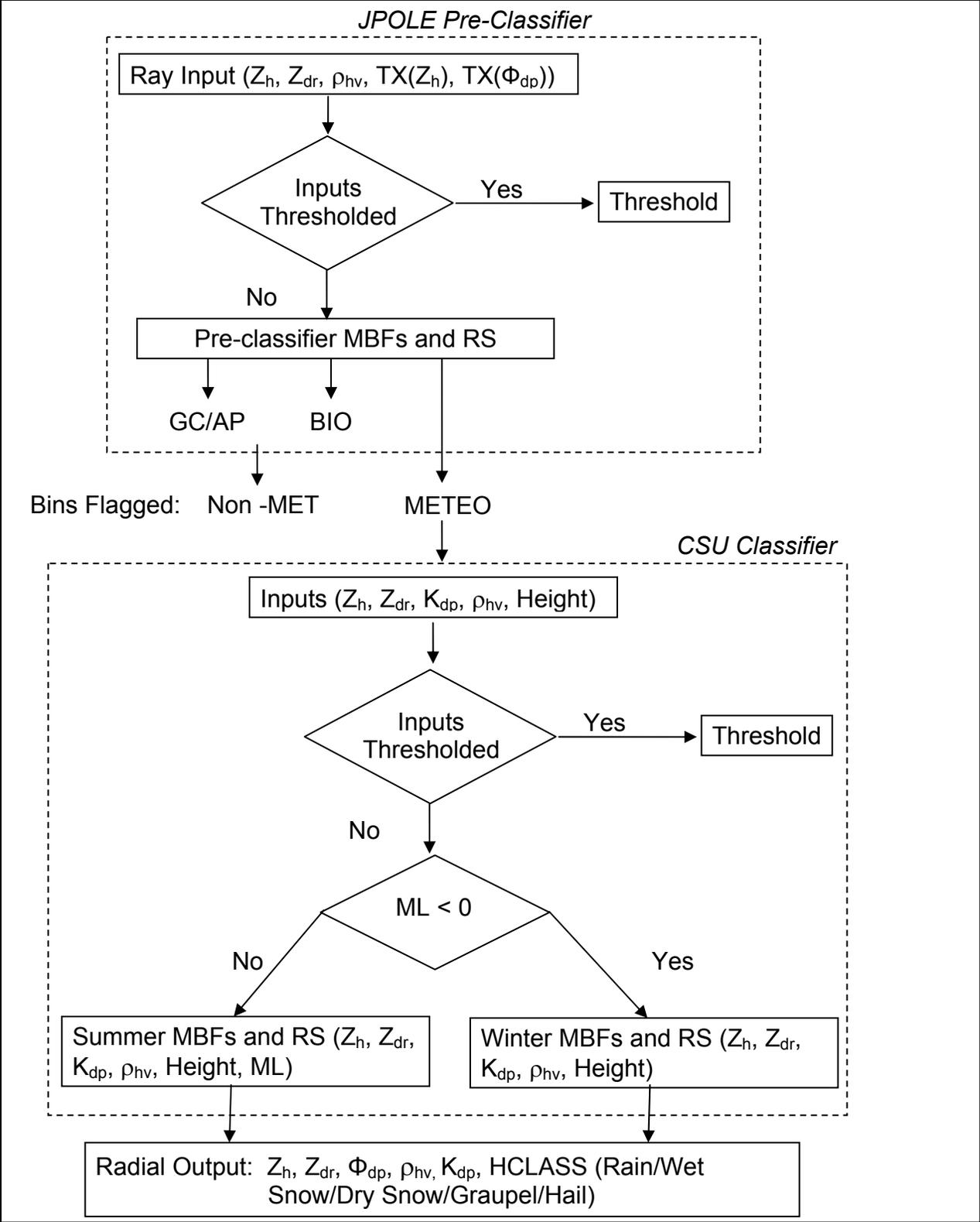
Figure 1. Hydrometeor classification processing steps within the signal processor.
