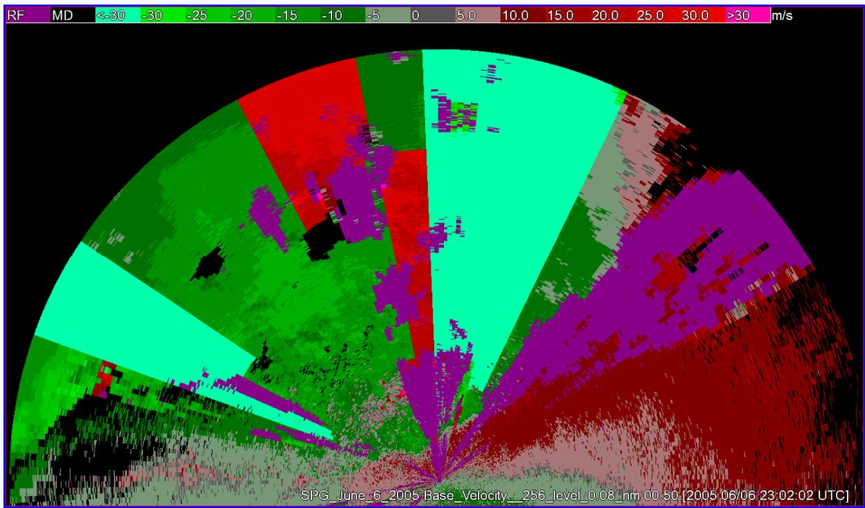
Fig. 1. Examples of velocity dealiasing errors from the SPG.
