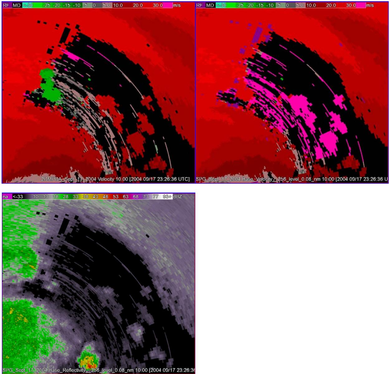
Fig. 4. Example of strongly biased velocity values associated with low reflectivities leading to a large-scale dealiasing error. Top-left shows 2DMPDA results and top-right shows SPG results.
