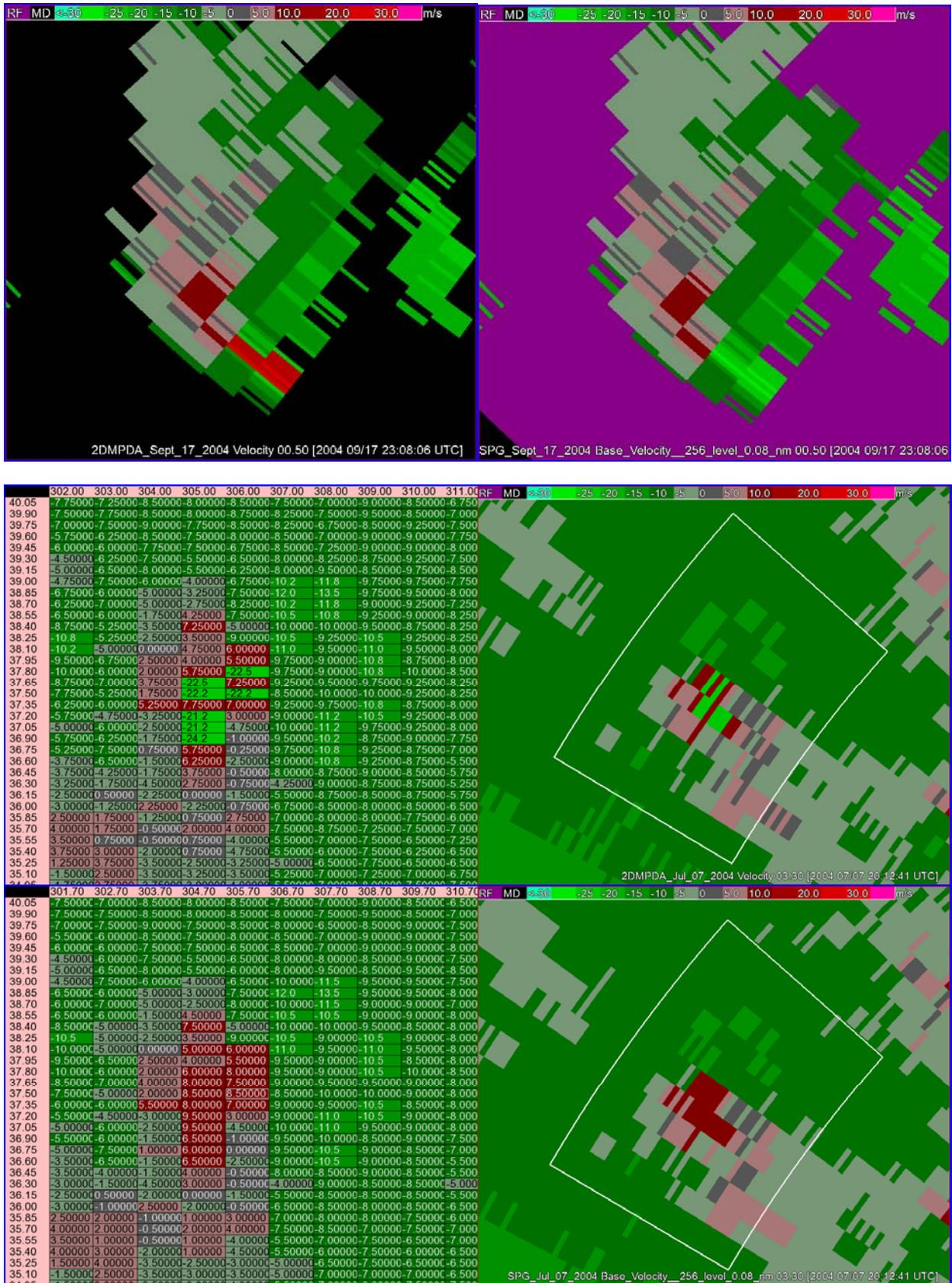
Fig. 3. Examples of velocity dealiasing errors made by the 2DMPDA (top-left and middle) involving storm-scale shear signatures, and the correct velocity data produced by the SPG (top-right and bottom).
